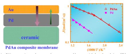
The hydrogen-selective PdAu composite membrane samples were prepared by sequential electroless plating of Pd and Au onto ceramic microfiltration support.
