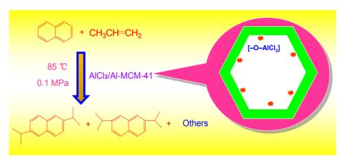
Alkylation of naphthalene with propylene can be carried out over AlCl<sub>3</sub>/Al-MCM-41 catalysts in a slurry bubble column reactor at 85 °C. The pore diameter influences the conversion of naphthalene and selectivity for 2,6-diisopropylnaphthalene.
