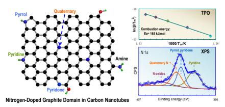
Functionalities on nitrogen-doped carbon nanotubes were identified and quantified, which is important for the clarification of structure-performance relationships in metal-free catalysis. A simple route to a closed cup-like carbon nanostructure is also reported.
