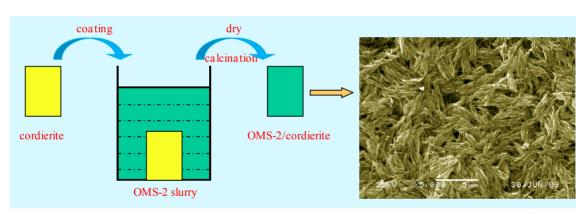
Manganese oxide octahedral molecular sieve (OMS-2)/cordierite monolithic catalysts were prepared by a coating method with common polymers as the binders. The catalyst prepared with 3%PVA-1799 showed higher catalytic activity for DME combustion and better reusability.
