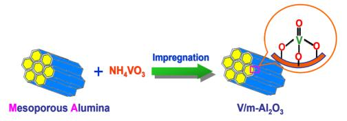
The impregnated vanadia catalyst supported on mesoporous alumina exhibits high performance for the oxidative dehydrogenation of propane to propene, because of highly dispersed vanadium active species and the weak acidity of the catalyst.
