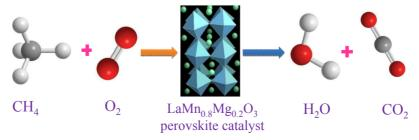
$LaMn_{0.8}Mg_{0.2}O_3$  perovskite catalyst prepared by the glycine-nitrate method and calcined at 700 °C shows the best activity for methane combustion. This is attributed to its smaller crystalline size, larger surface area, and more  $Mn^{4+}$  cations on its surface.
