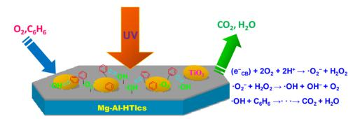
Under UV light irradiation, a large number of 'OH was generated on the surface of Mg-Al-HT (hydrotalcite-like compound) TiO<sub>2</sub> heterocompounds, which is the key factor in the oxidation of benzene.
