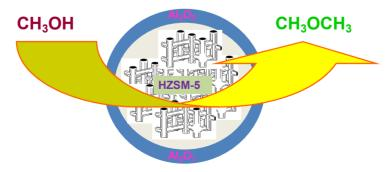
Combined  $Al_2O_3$ -HZSM-5 solid acids exhibit higher methanol dehydration activity and higher stability at lower temperature (235 °C) and a higher LHSV (30 h<sup>-1</sup>).
