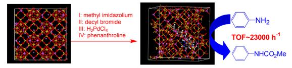
The integration of a free palladium complex and an ionic liquid molecule into the super-cage of a NaY zeolite to form an effective catalytic site was developed by a molecular self-assembly/ship-in-bottle method. Much higher catalytic activity was achieved for the carbonlytion of aniline with much lower amounts of the ionic liquid and palladium complex.
