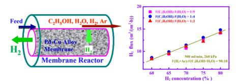
Pd-Cu alloy membrane exhibited good performance in a membrane reactor with H<sub>2</sub>-Ar-C<sub>2</sub>H<sub>5</sub>OH-H<sub>2</sub>O modeling mixture for steam reforming of ethanol and showed potential application for pure hydrogen production from the reforming reaction.
