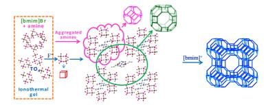
The LTA type framework with cage structure was ionothermally synthesized through the synergetic effect of the introduced amine of an aggregated state together with the cation of the ionic liquid.
