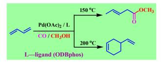
Carboxylation of 1,3-butadiene catalyzed by Pd(OAc)<sub>2</sub>/(oxydi-2,1- phenylene)bis(diphenylphosphine) catalyst in the presence of CO and MeOH was carried out, reaching 90.4% conversion of 1,3-butadiene and 91.6% selectivity for methyl 3-pentenoate, while dimerization occurred at 200 °C to form 4-vinyl-1-cyclohexene in 96% yield.
