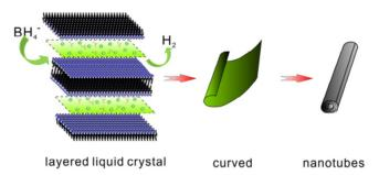
Noncrystalline alloy nanotubes were prepared using NaBH<sub>4</sub> to reduce the transition metal ions located in the layer structure of lytropic liquid crystals of nonionic/anionic mixed surfactants. These nanotubes exhibit high efficiency for catalytic hydrogenation because of their characteristics of structure and morphology.
