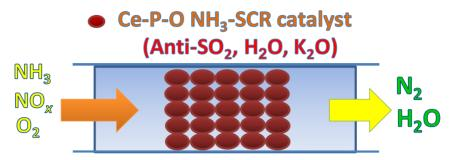
The new highly active Ce-P-O catalyst for the selective catalytic reduction (SCR) of NO with NH<sub>3</sub> in the presence of excess O<sub>2</sub> was developed, and the catalyst was resistant to steam and SO<sub>2</sub>.
