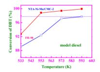
Mesoporous carbon supported Co-Mo-S and Ni-Mo-S catalysts are shown to exhibit high activity for the hydrodesulfurization of thiophene in a model gasoline and of dibenzothiophene (DBT) in a model diesel, respectively.
