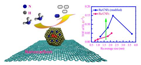
Ru/CNFs and Ru/CNTs catalysts were prepared and used for ammonia decomposition. Surface defects and surface oxygen complexes on the CNFs remarkably enhance the activity of the Ru catalysts.
