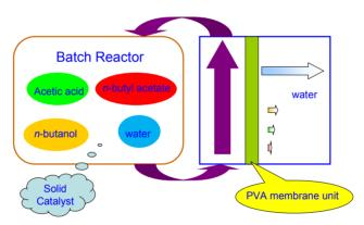
An accurate mathematical model was developed for esterification in a batch reactor coupled with pervaporation by taking into account the non-ideal thermodynamic behavior of the components involved in the reaction.
