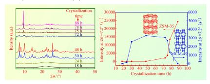
In a hexamethyleneimine-cyclohexamine system, MCM-49 was obtained first, then MCM-49/ZSM-35 composite zeolites were gradually formed with increasing ZSM-35 content upon the crystallization time, and finally ZSM-35 was produced.
