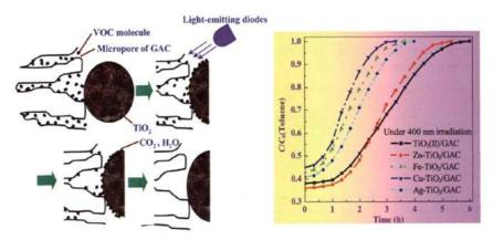
UV wavelength light emitting diodes were used for the adsorption photocatalytic removal of volatile organic compounds and of granular activated charcoal (GAC) that was impregnated with a TiO<sub>2</sub> photocatalyst or with TiO<sub>2</sub>/co-catalysts, which resulted in enhanced removal efficiency.
