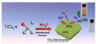
A green solvothermal route is proposed for the synthesis of F/TiO<sub>2</sub> nanocrystals with exposed (001) facets and with high photocatalytic activity induced by photogenerated holes, •OH, and •O<sub>2</sub> active species.
