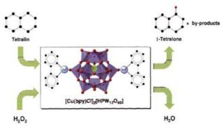
Cu(II) bipyridine and phenantroline complexes were immobilized on  $H_3PW_{12}O_{40}$  polyoxometalate and used as heterogeneous catalysts for the selective oxidation of tetralin. A conversion of 16% with 83% selectivity for 1-tetralone and 2-tetralone were obtained with the  $[Cu(1,10\text{-phen})Cl][H_2PW_{12}O_{40}]$  complex.
