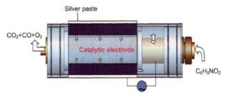
Purification of air streams containing dilute nitrobenzene was carried out in a dielectric barrier discharge reactor with a modified inner electrode. The  $CoO_x$  modified inner electrode gave a better performance with complete oxidation of 100 ppm of nitrobenzene at input energy < 300 J/L.
