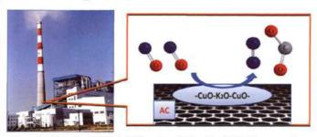
NO was effectively reduced by activated carbon over a Cu-K-O catalyst. Adding K to CuO/AC promoted the reaction between the surface carbon active sites and the surface oxygen species.
