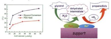
The addition of Re increased the acid sites of Ru-Re/SiO<sub>2</sub>, which increased the activity for glycerol hydrogenolysis. A synergy of ReO<sub>x</sub> acid sites and Ru<sup>0</sup> metal sites gave the high activity.
