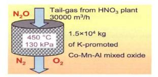
A K-promoted Co-Mn-Al mixed oxide catalyst derived from a layered double hydroxide was used to estimate the size of a N<sub>2</sub>O decomposition reactor for use in exhaust gas purification in a nitric acid production unit.
