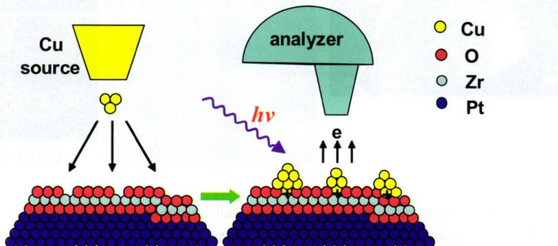
Cu grows two-dimensionally on ZrO<sub>2</sub>(111)/Pt(111) up to 0.15 ML at 300 K, followed by three-dimensional growth. At low coverages, Cu(I) state appears. Above 1 ML, Cu becomes metallic state.
