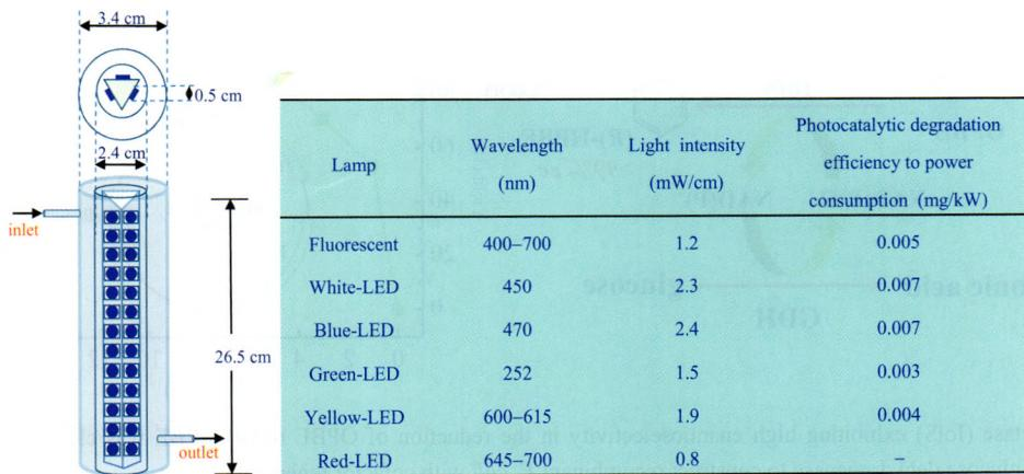
The use of chips of visible light emitting diodes to irradiate an annular reactor coated with a nitrogen doped titania catalyst to decompose gaseous aromatic compounds was studied.
