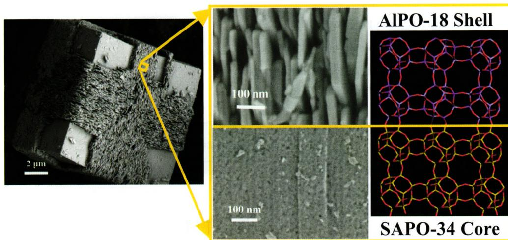
The core-shell SAPO-34/AlPO-18 molecular sieves were hydrothermally synthesized through the epitaxial growth of AlPO-18 shell induced rationally by the microstructure on the SAPO-34 external surface.
