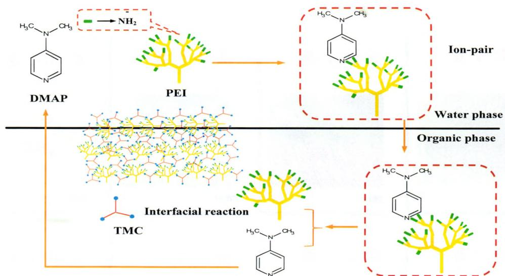
The promoting effect of 4-dimethylaminopyridine (DMAP) on the interfacial polymerization between trimesoyl chloride (TMC) and hyperbranched polyethylenimine(PEI) to prepare reverse osmosis membrane was investigated. The rejection against NaCl of PEI/TMC reverse osmosis composite membrane was improved from 45.2% to 85.4%.
