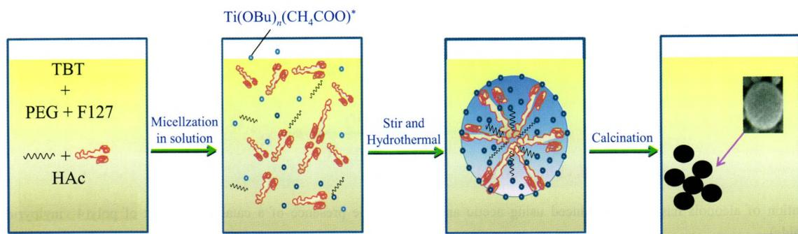
Mesoporous TiO<sub>2</sub> (MS-TiO<sub>2</sub>) spheres were synthesized with double surfactant (PEG and F127) as templates, which showed higher reliability than single template.
