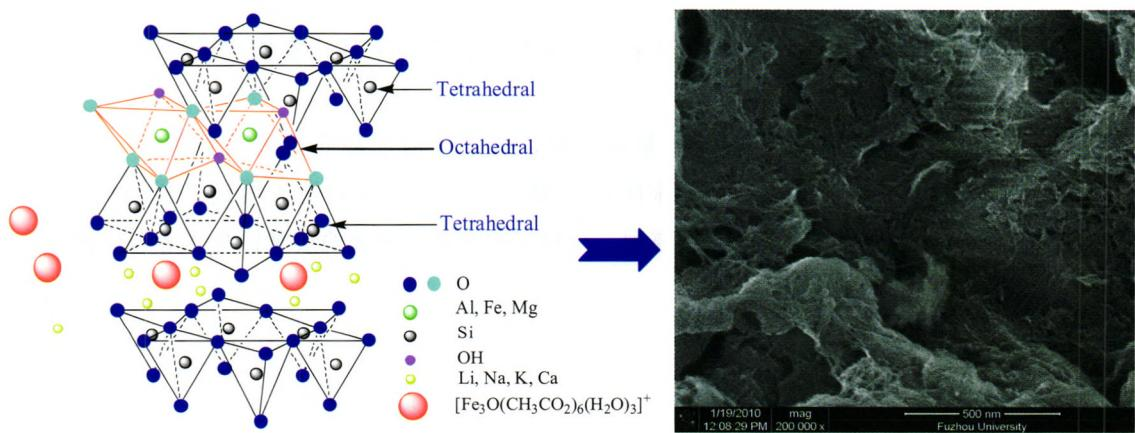
A large iron cluster was intercalated into the lays of montmorillonite via a facile cation exchange method. The SEM image shows that a few amorphous nano-fibre iron oxides were anchored on the surface of the intercalated montmorillonite.
