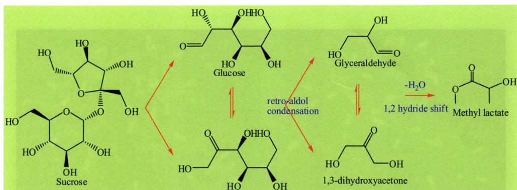
Biomass-derived carbohydrates were used as feedstock and methyl lactate was obtained in higher yield of 40%. Catalysts used in this work are easy synthesis, operational simplicity, reusability, and safe handling.
