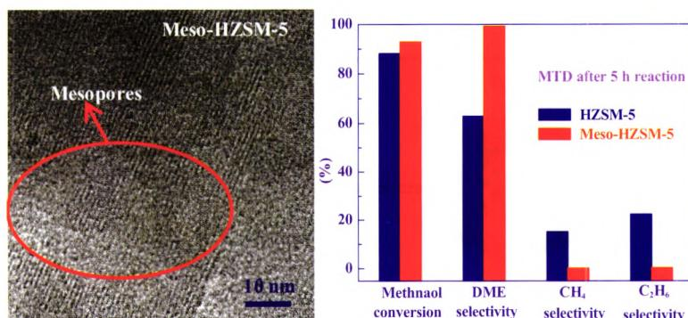
The synthesized hierarchical mesoporous HZSM-5 zeolites exhibited better catalytic activity than conventional HZSM-5, indicating that hierarchical mesopores play an important role in the methanol to dimethyl ether process.
