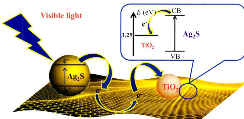
This paper presents the research of synthesized  $\text{Ag}_2\text{S}$ -graphene/ $\text{TiO}_2$  by the sonochemical method. The generation of reactive oxygen species was detected through the oxidation reaction from 1,5-diphenyl carbazide to 1,5-diphenyl carbazone.
