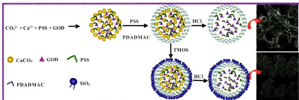
Glucose oxidase (GOD) was immobilized in organic-inorganic composite microcapsules using a combination of layer-by-layer assembly and biomimetic mineralization. The encapsulated GOD exhibited distinct advantages in terms of thermal, pH, and operational stabilities.
