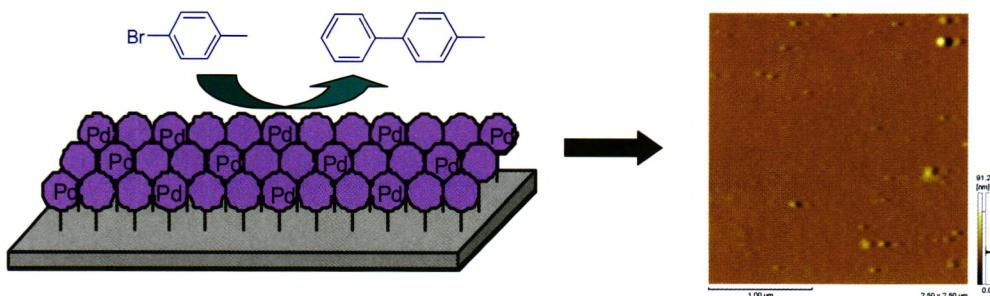
The amphiphilic cyclopalladated aryl imine catalysts were successfully transferred on the solid slides and can be used for the Suzuki reactions.
