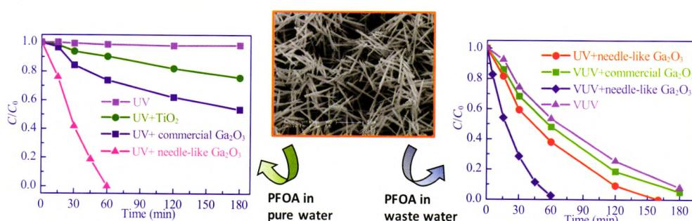
In combination with 185 nm vacuum UV irradiation, needle-like Ga<sub>2</sub>O<sub>3</sub> showed high efficiency for the removal of trace perfluorooctanoic acid (PFOA) in wastewater where the decomposition of PFOA by other catalysts is usually inhibited by coexisting natural organic matters.
