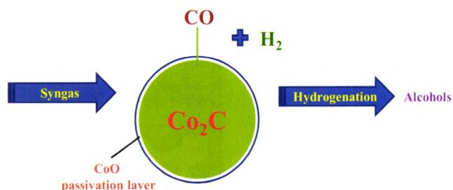
Co<sub>2</sub>C was prepared by carburizing Co with CO. The prepared Co<sub>2</sub>C samples were composed of a bulk Co<sub>2</sub>C phase and an outer CoO passivation layer. Co<sub>2</sub>C could adsorb CO, which was hydrogenated into alcohol.
