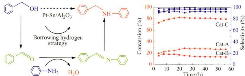
Pt-Sn/Al<sub>2</sub>O<sub>3</sub> catalysts with highly dispersed Pt particles, weak acid sites, acid distributions, and large pore volumes and pore size distributions have excellent catalytic performance in the synthesis of secondary amines.
