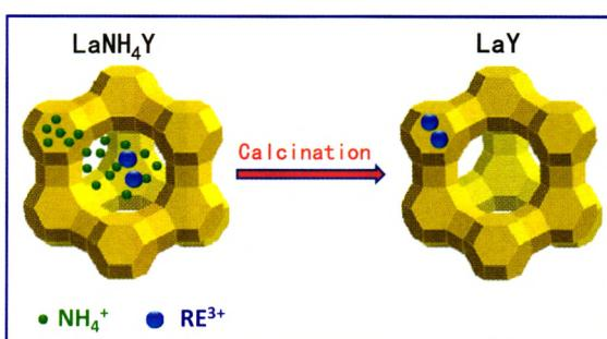
Lanthanum cations are initially distributed in supercages and then migrate to Si<sup>4+</sup> located inside sodalite cages during heating and dehydration.
