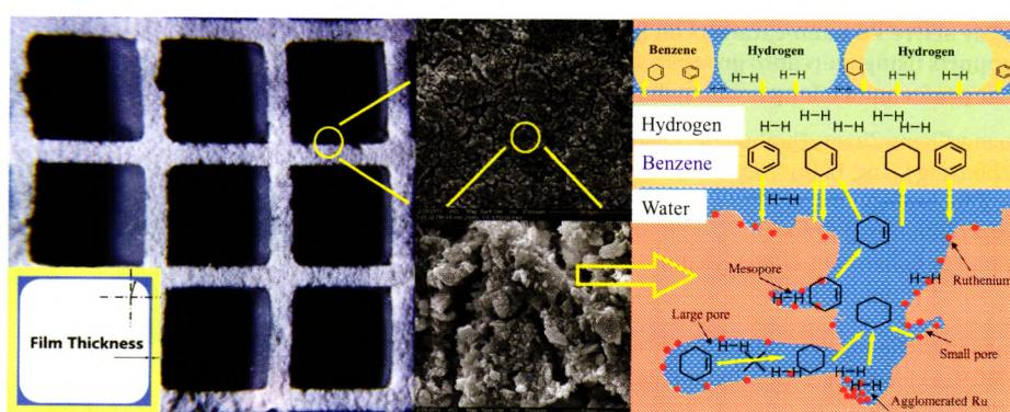
Novel egg-shell-like Ru/Al<sub>2</sub>O<sub>3</sub>-ZrO<sub>2</sub>-NiO/cordierite monolithic catalysts with tailored pore structure are fabricated. Mesopores and low pore volume are needed to obtain a reasonable yield of cyclohexene using the monolithic catalysts with a low concentration of ZnSO<sub>4</sub> solution.
