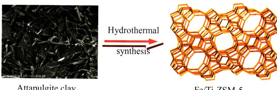
Fe/Ti-ZSM-5 zeolite was synthesized from treated attapulgite (ATP) mineral. Compared with conventional ZSM-5 zeolite, Fe/Ti-ZSM-5 exhibits relatively high yields of light olefins in the catalytic cracking of Canadian light gas oil.
