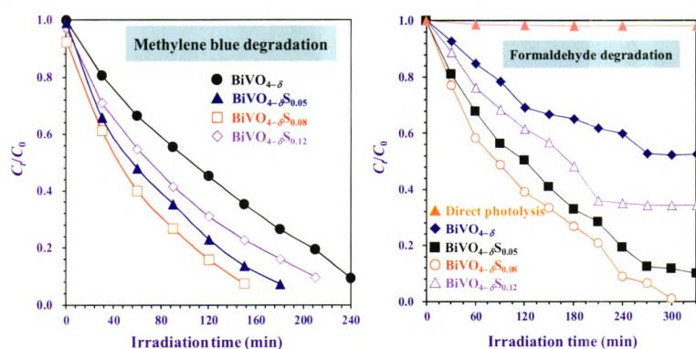
Porous BiVO<sub>4-δ</sub> and BiVO<sub>4-δ</sub>S<sub>σ</sub> are fabricated using dodecylamine-assisted alcohol-hydrothermal strategy. The higher O<sub>ads</sub> concentration and lower bandgap energy account for excellent photocatalytic performance of BiVO<sub>4-δ</sub>S<sub>0.08</sub> for methylene blue and formaldehyde degradation.
