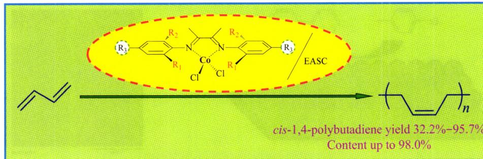
A series of cobalt(II) complexes ligated by  $\alpha$ -diimine have been synthesized and characterized. The catalyst system [ $\alpha$ -diimine]CoCl<sub>2</sub>/EASC shows high catalytic activity and *cis*-1,4 selectivity (up to 98%) for 1,3-butadiene polymerization.
