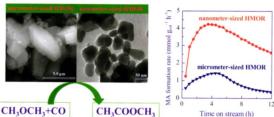
Nanometer-sized H-mordenite (HMOR) showed a much higher reaction rate and stability than micrometer-sized HMOR, resulting from the improvement of molecule transportation efficiency by reducing the crystalline size.
