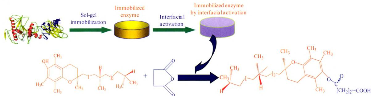
Interfacial activated *Candida rugosa* lipase encapsulated in sol-gel materials was prepared and used to synthesize vitamin E succinate.
