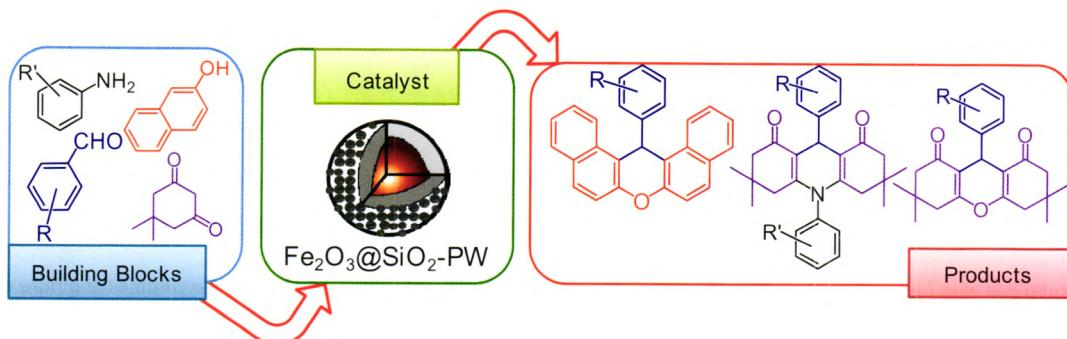
12-Tungstophosphoric acid (PW) catalysts supported on aerosil silica and silica-coated  $\gamma$ - $\text{Fe}_2\text{O}_3$  nanoparticles ( $\text{Fe}_2\text{O}_3@\text{SiO}_2-\text{PW}$ ) were prepared and characterized. These catalysts were used for the aqueous syntheses of 1,8-dioxo-9,10-diaryldecahydroacridines and xanthene derivatives, which are biologically interesting compounds.
