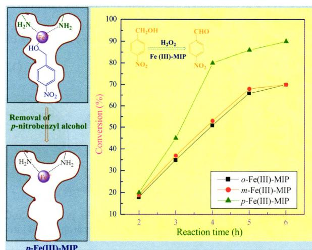
A series of molecularly imprinted polymers (MIPs) containing the equal amount of iron(III) were found to be the specific substrate recognition catalysts in the oxidation of substituted benzyl alcohol in water.
