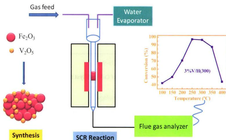
A series of highly dispersed  $\text{V}_2\text{O}_5$ /hematite (V/H) catalysts were prepared by the impregnation of  $\text{V}_2\text{O}_5$  on goethite, which were highly efficient for the selective catalytic reduction of NO with  $\text{NH}_3$ .
