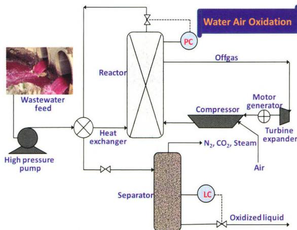
Wet air oxidation (WAO) is one of the most economically and technologically viable advanced oxidation processes for dye wastewater. The wide studies on WAO of dye wastewater began from 1995. Recent studies focused on real wastewaters.
