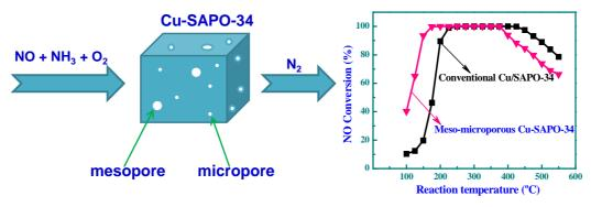
H-Cu-SAPO-34 catalysts with full mesopores and excellent performance in low-temperature NH<sub>3</sub>-SCR of NO have been controllably synthesized via a one-pot hydrothermal crystallization method. Importantly, the formation of micro-mesopores in the Cu-SAPO-34 catalysts decreases diffusion resistance and greatly improves the accessibility of reactants to the catalytic active sites.
