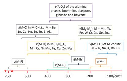
Far infrared spectroscopy complements the application of mid-infrared, near-infrared spectroscopy with the advantage of capable of measuring these typical lower energy vibration modes accurately.
