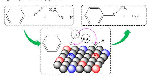
Under catalysis of  $KH_2PO_4/Al_2O_3$ , phenol and methanol was activated by K and Al sites respectively. Anisole yield decreased with increasing space velocity, increased with increasing methanol fraction, and appeared a maximum value with increasing temperature.
