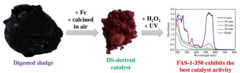
Digested sludge-derived photo-Fenton catalysts were synthesized via a facile three-step method. The catalyst produced using ferrous ammonium sulfate in conjunction with a calcination temperature of  $350\,^{\circ}\text{C}$  exhibits the best catalytic activity because of its faster reaction rate and lower Fe leaching.
