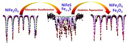
Ferrite adsorbents can be synthesized using a microwave assisted combustion method, yielding a high desulfurization capability. Mössbauer spectroscopy was used to characterize the ferrites. The adsorbents were successfully regenerated under oxidizing conditions.
