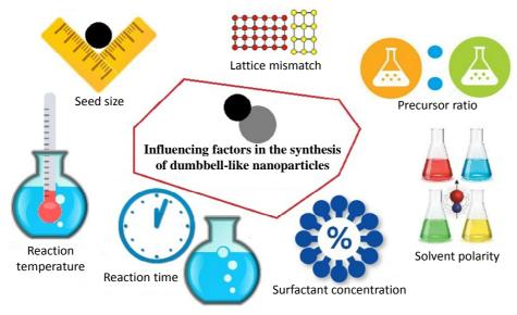
This article reviews some significant factors in the synthesis of dumbbell-like nanoparticles, including seed size and size ratio, reaction temperature and time, solvent polarity, precursor ratio, lattice mismatch, and surfactant concentration.
