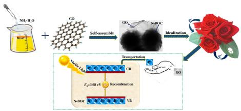
Microspheres of graphene oxide (GO) coupled to N-doped (BiO) $_2$ CO $_3$  showed improved photocatalytic activity compared to pure BOC and N-BOC, which was due to the high electron-withdrawing ability and conductivity of GO and improved visible light harvesting ability of the 3D hierarchical architecture.
