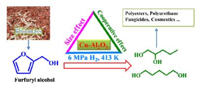
The size and cooperative effects of highly dispersed Cu nanoparticles and an acidic  $Al_2O_3$  support are significant factors affecting the selective hydrogenolysis of furfuryl alcohol to 1,2- and 1,5-pentanediols over Cu-Al<sub>2</sub>O<sub>3</sub> catalysts.
