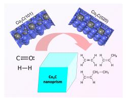
$Co_2C$  nanoprisms with the exposed facets of (101) and (020) exhibit strong facet effect for syngas conversion with high selectivity for the production of lower olefins, while generating little methane.
