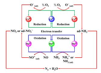
Electron interaction between  $MnO_x$  and  $CeO_2$  is influenced by the preparation methods, which can improve the physicochemical properties of  $MnO_x$ - $CeO_2$  catalysts, and promote the adsorption/activation of reactant molecules to result in excellent catalytic performance.
