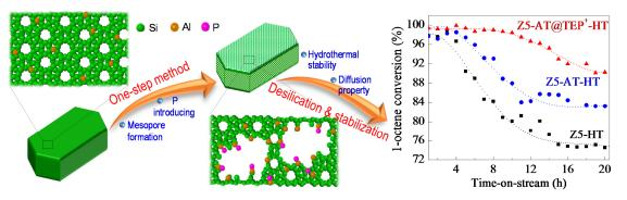
Hierarchically porous ZSM-5 with high hydrothermal stability was obtained by a one-step post-synthesis treatment involving simultaneous controlled desilication and phosphorous modification. The prepared catalyst displayed prolonged catalytic activity and stability toward hydrocarbon cracking.
