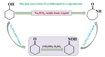
Na<sub>2</sub>WO<sub>4</sub>-acidic ionic liquid was used as a simple, ecofriendly, recyclable and efficient catalytic system in the one-pot synthesis of  $\varepsilon$ -caprolactam from cyclohexanol, hydrogen peroxide, and hydroxylamine.
