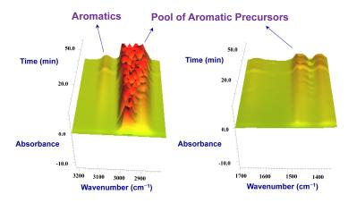
An *operando* dual-beam Fourier transform infrared spectrometer was developed using a facile method, and was successfully used to characterize the dynamic processes in isobutene aromatization over nano-sized HZSM-5 zeolite under real reaction conditions.
