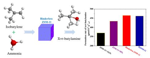
A shaped binderless ZSM-11 catalyst was prepared by the dry-gel conversion technique and showed superior performance in isobutene animation reaction.
