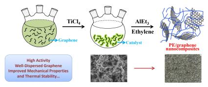
A facile coagglomeration method for preparing graphene/MgCl<sub>2</sub>-supported Ziegler-Natta catalyst was reported. After in-situ ethylene polymerization, the resultant polyethylene/graphene nanocomposites exhibited enhanced thermal stability and mechanical properties than neat polyethylene.
