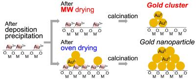
Small gold nanoparticles and clusters could be deposited on metal oxides by deposition-precipitation followed by microwave drying and calcination. The MW drying can be applied to several metal oxides regardless of the MW absorption efficiency.
