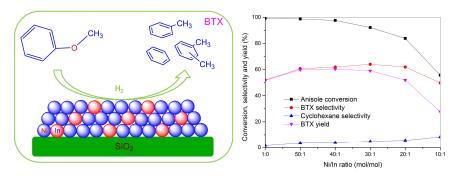
In the hydrodeoxygenation of anisole, used as a bio-oil model compound, the activities of Ni-In/SiO<sub>2</sub> bimetallic catalysts in benzene ring hydrogenation and C–C bond hydrogenolysis were much lower than that of Ni/SiO<sub>2</sub>, leading to higher selectivities for BTX and cyclohexane.
