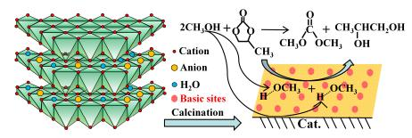
Solid base catalysts derived from Ca-M-Al (M = Mg, La, Ce, Y) layered double hydroxides were found to be both recyclable and highly active during dimethyl carbonate production under heterogeneous conditions.
