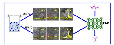
The crystallization behavior of FER zeolite is closely related to the crystallization temperature, with well-crystallized FER zeolite showing good catalytic performance in 1-butene skeletal isomerization.
