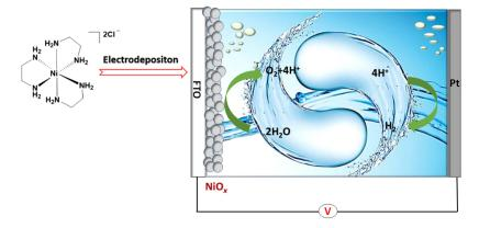
A  $NiO_x$  film was prepared by electrodeposition of a nickel-based molecular precursor at pH = 11. The thin film exhibits high activity for electrochemical water oxidation.
