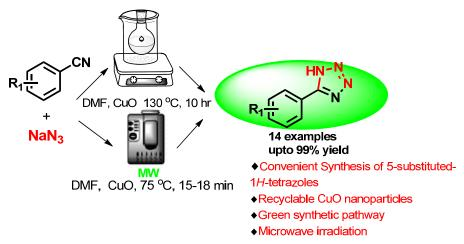
We demonstrate that practical, simple, efficient and recyclable CuO nanoparticles can catalyze the (3+2) cycloaddition of nitriles and  $NaN_3$  to synthesize 5-substituted-1*H*-tetrazoles using microwave irradiation.
