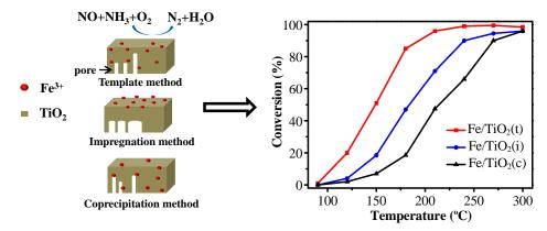
The Fe-TiO $_2$  catalyst synthesized by a F127-assisted process showed the uniform mesopore structure, the strong interaction between Fe and Ti, and the excellent SCR activity in mid-temperature region with the comparation of catalysts prepared by traditional impregnation and coprecipition methods.
