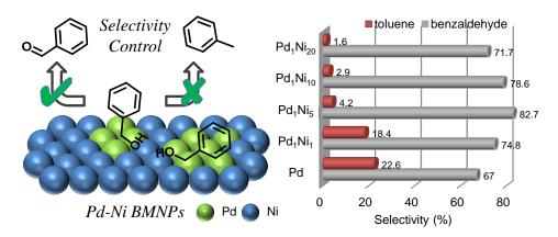
Supported Pd-Ni bimetallic nanoparticles prepared through a solid-state alloying method can enhance the selectivity towards benzaldehyde by effective suppression of toluene formation in a solvent-free benzyl alcohol oxidation reaction.
