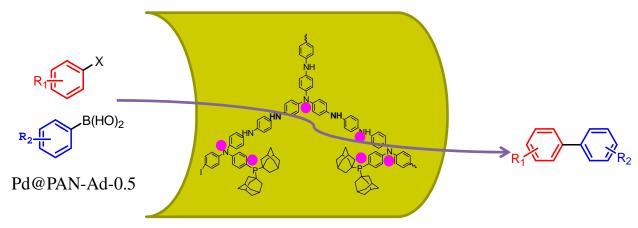
Palladium nanoparticles supported on cross-linked polyaniline with bulky phosphorus-based ligands were developed as highly efficient catalysts for the Suzuki-Miyaura reaction of aryl chlorides and bromides with phenylboronic acids.
