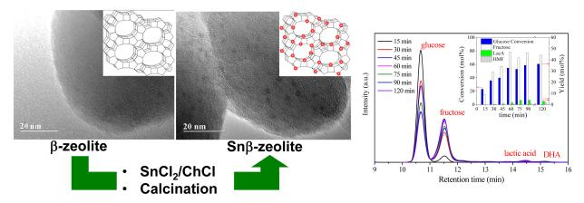
$Sn-\beta$ -zeolite prepared by immobilization of  $SnCl_2/ChCl$  followed by calcination showed good activity and high selectivity for glucose-fructose isomerization.
