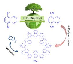
Covalent triazine-based frameworks were prepared from the corresponding dicyano monomers by cyanation of aryl bromides with nontoxic potassium hexacyanoferrate(II) in the presence of palladium acetate.
