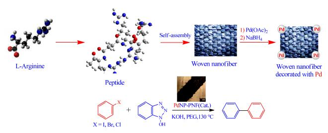
Pd nanoparticles supported on peptide nanofibers (PdNP-PNF) represent unique catalytic activity for the phenylation of aryl halides by hydroxybenzotriazole as new phenylating agent under green reaction conditions.
