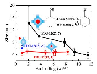
FDU-12 having a sub-5-nm entrance size stabilizes gold nanoparticles over a controlled narrow size distribution across a wide loading concentration during heat-treatment, thus optimizing their catalytic properties in the gas-phase selective oxidation of cyclohexanol.
