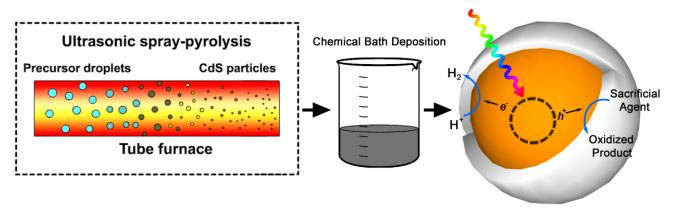
CdS/ZnS core-shell heteromicrostructures with optimized amount of ZnS loaded as shell were synthesized by a simple two-step method. Surface treatments further improve their photocatalytic activities and stabilities. This method demonstrates a promising low-cost synthesis of core/shell microstructures.
