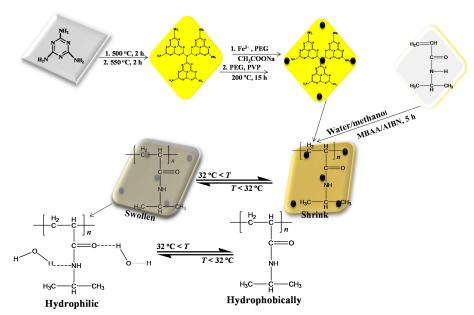
A stable and magnetic  $PNIPAM/Fe_3O_4/g$ - $C_3N_4$  photocatalyst was fabricated by a hydrothermal method and thermal photoinitiating technology. Its activity could be modulated by temperature, showing promise for use in intelligent catalysis.
