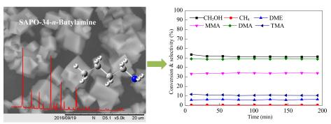
n-Butylamine was used as a template to synthesize SAPO-34 with excellent shape-selective catalytic performance in the methanol amination reaction.
