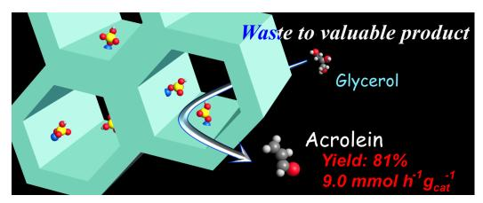
Mesoporous sulfated zirconia-silica catalyst bearing only Brønsted acid sites selectively converts glycerol to acrolein in gas phase at 523 K. Mild acid strength, absence of Lewis acid sites and large pore benefit the reaction.
