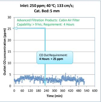
Highly active Pt-Ceria/silica catalyst for low temperature CO oxidation in humid air has been developed. Effect of catalyst preparation variables was studied and the activity maintenance of the catalyst for different applications was investigated.
