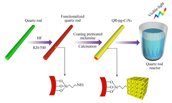
Porous g- $C_3N_4$  and supported porous g- $C_3N_4$  were fabricated for the first time by a simple precursor pretreatment strategy and applied in organic-pollutant degradation, hydrogen evolution, and simultaneous hydrogen evolution with organic-pollutant degradation under visible-light irradiation.
