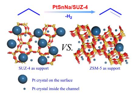
The new catalyst PtSnNa/SUZ-4 was found to be superior to PtSnNa/ZSM-5 during propane dehydrogenation, at least partly because Pt particles on the PtSnNa/SUZ-4 are primarily dispersed over its external surface and so are not deactivated by carbon deposition.
