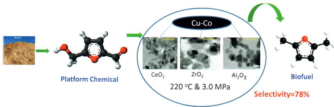
The present study explored the use of non-noble, environmentally benign, bimetallic copper-cobalt catalysts in the selective production of 2,5-dimethylfuran via 5-hydroxymethylfurfural hydrogenolysis.
