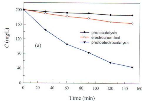
We have synthesized and fully characterized BiVO<sub>4</sub> on FTO substrate. Electrochemical, photochemical and photoelectrochemical oxidation of chlorate was investigated. High rate constant of chlorate oxidation was obtained by photoelectrochemical method, as compared to other two methods.
