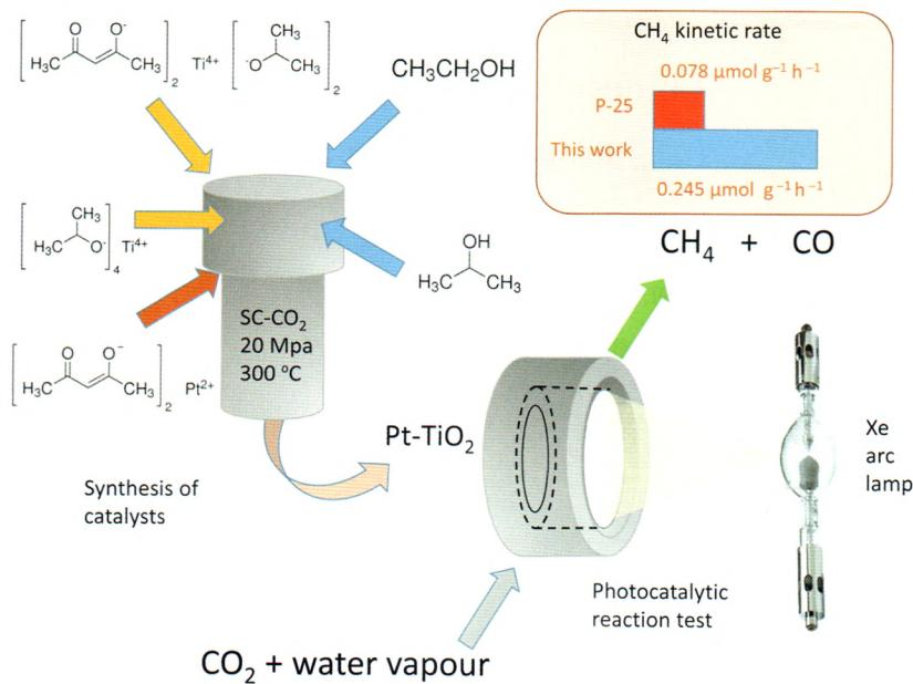
The catalytic properties of Pt/TiO<sub>2</sub> particles can be tuned by simply changing operating parameters like the type of titania precursor and/or hydrolysis agent when their hydrothermal formation reaction is accomplished in supercritical CO<sub>2</sub>. The synthesised particles exhibit superior performance to that of a commercial catalyst in the photocatalytic reduction of CO<sub>2</sub> to methane.
