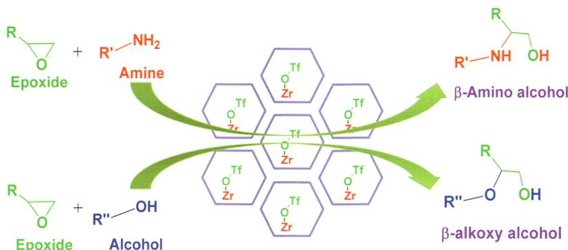
We report the synthesis of zirconium triflate grafted mesoporous SBA-15 ( $ZrTf/S$ ) using a simple one-pot-two-step synthesis.  $ZrTf/S$  showed excellent activity for ring opening of epoxides by various amines and alcohols under ambient conditions.
