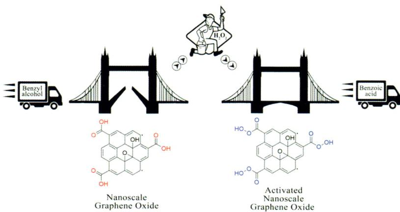
Nanoscale graphene oxide sheets as active graphene-based carbocatalysts with peroxidase-like activity convert to peroxybenzoic acid in the presence of  $H_2O_2$ , and act as efficient catalysts for oxidation of benzylic alcohols.
