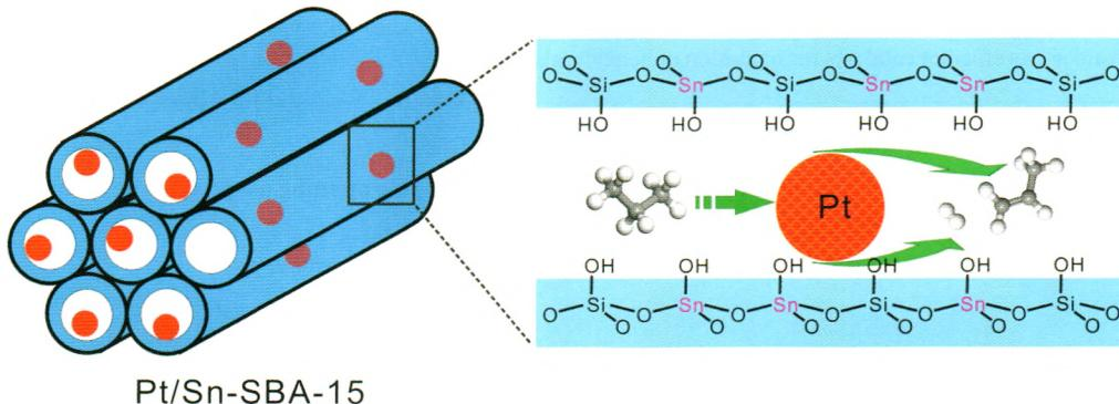
A facile one-pot method was used to synthesize ordered mesoporous Sn-SBA-15-supported Pt catalysts with stable SnO<sub>x</sub> species and enhanced promotion by Sn species. The materials gave excellent catalytic performance and good resistance to coking in propane dehydrogenation.
