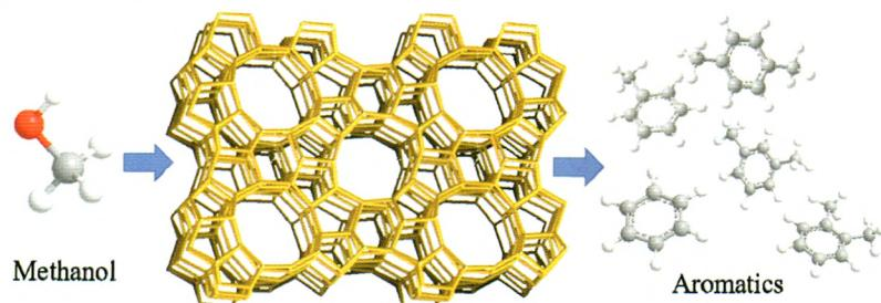
The effect of H-ZSM-5 crystal size on the methanol-to-aromatics reaction has been systematically investigated. Nano-sized hierarchical H-ZSM-5 shows enhanced catalytic activity attributed to the presence of auxiliary meso- and macropores and larger external surface areas.
