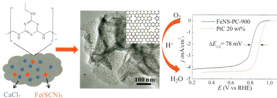
Fe, N, S-doped porous carbon was synthesized by direct carbonization of a mixture of melamine formaldehyde resin and  $\text{Fe}(\text{ScN})_3$  using  $\text{CaCl}_2$  as a template. The porous carbon showed high activity and durability in the oxygen reduction reaction.
