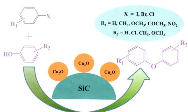
A Cu<sub>2</sub>O/SiC heterogeneous catalyst was highly active in Ullmann-type C–O cross-coupling reactions of aryl halides and phenols, with a turnover frequency of up to 1136 h<sup>-1</sup>, and showed general applicability to Ullmann cross-coupling reactions.
