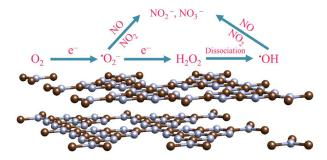
Using a closely combined theoretical and experimental approach, the reactive oxygen species behavior on g- $C_3N_4$  for effective NO removal and the reaction mechanism at the atomic level were clarified, which enriches the understanding of ROS in photocatalytic environmental remediation.
