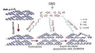
The periodic oxidation and exfoliation on g- $G_3N_4$  photocatalysts under long-time DBD treatment is reported. Further, chemical and physical changes on g- $G_3N_4$  influence the photocatalytical activities.
