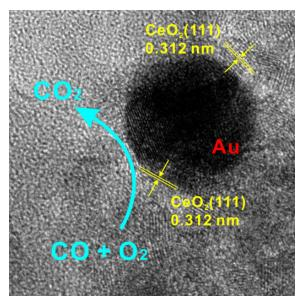
It has been successfully synthesized a  $CeO_x@Au/SiO_2$  catalyst with both high activity and excellent durability in CO oxidation. Key to the success is to construct abundant Au- $CeO_x$  interfaces by modification of Au nanoparticles with  $CeO_x$  nanocrystals.
