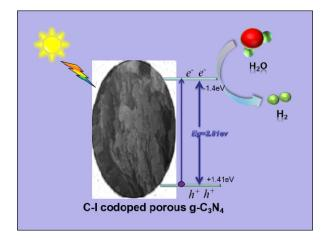
C-I co-doped porous  $g-C_3N_4$  synthesized from two-step thermal polymerization method was demonstrated as a stable photocatalyst for  $H_2$  evolution under visible light irradiation.
