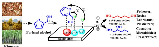
The synergism between balanced Cu<sup>0</sup> and CoO sites played a critical role in achieving a high yield of PeDs with high 1,5-/1,2-pentanediol selectivity ratio during the hydrogenolysis of biomass-derived furfuryl alcohol.
