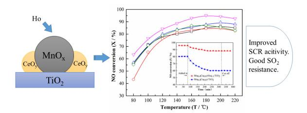
Ho can be an effective doping element for improving the low-temperature SCR performance and the SO<sub>2</sub> resistance of Mn-Ce/TiO<sub>2</sub> catalyst.
