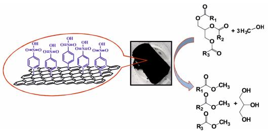
Graphene-based acidic catalysts exhibit a high performance and good stability in the transesterification reaction, which make them promising catalysts for biodiesel fuel production.
