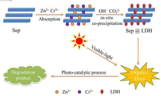
Sep@LDH composites were successfully synthesized by a facile *in situ* co-precipitation method and exhibited high photocatalytic performances towards the degradation of co-existing MO and MB under visible-light irradiation, where Sep was an excellent carrier.
