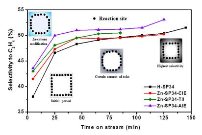
The Zn cation-modified SAPO-34 catalysts with core-shell like structure favor the quick establishment of catalytic environment for effective MTO reaction with the selective production of ethylene via introducing extra diffusion limitation for the higher hydrocarbon products.
