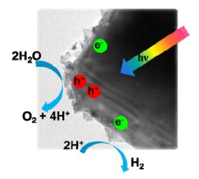
Self-distribution of redox dual-cocatalysts on semiconductor surface can be achieved by photogenerated electrons and holes. This strategy promotes the photocatalytic activity to a high level, which will be benefit for solar energy conversion system.
