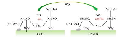
$NH_3$ - $NO/NO_2$  SCR reaction routes on CeTi and CeWTi catalysts. Addition of  $WO_3$  provides more acid sites which accelerate the reaction between  $NH_4NO_3$  and NO to get a superior low-temperature activity.
