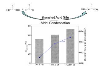
Brönsted acid was an active site for aldol condensation reaction of DMM and MAc to produce MA and AA. The selectivity of MA and AA increased with the concentration of Brönsted acid.
