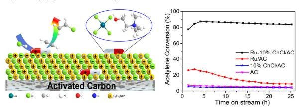
The supported Ru(III)-ChCl/AC catalyst system, where ChCl provides an environment for the ChRuCl<sub>4</sub> to be stabilized as Ru(III), shows superior activity and stability in acetylene hydrochlorination.
