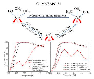
The redox cycle of  $Cu^*$  and octahedrally coordinated  $Cu^{2*}$  significantly affected the high hydrothermal stability and resistance to hydrocarbons of Cu–Mn/SAPO-34.
