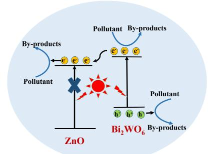
The  $Bi_2WO_6/ZnO$  composite photocatalyst was employed to degrade methylene blue and tetracycline. Under visible light, the  $Bi_2WO_6/ZnO$  composite shows excellent photocatalytic activity for methylene blue and tetracycline within a short irradiation time.
