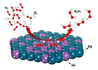
Highly selective Pd-Sb/ $TiO_2$  bimetallic catalysts for the direct synthesis of  $H_2O_2$  were obtained, and the addition of Sb increased the isolated Pd sites, which are favorable for  $H_2O_2$  formation.
