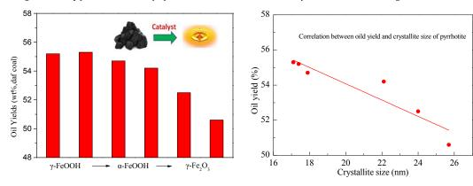
Precursors consisting of iron–oxygen compounds with  $\gamma$ -FeOOH or  $\alpha$ -FeOOH crystalline phases that are readily transformed into fine crystallites of pyrrhotite exhibit superior catalytic activity during direct coal liquefaction.
