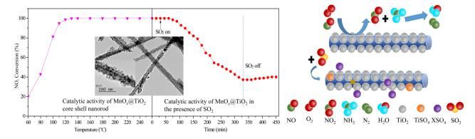
This work reports a novel  $MnO_x@TiO_2$  core–shell nanorod catalyst, which exhibits high activity and enhanced  $SO_2$  tolerance for the low-temperature selective catalytic reduction of  $NO_x$  with  $NH_3$  due to the protective effect of the  $TiO_2$  shell.
