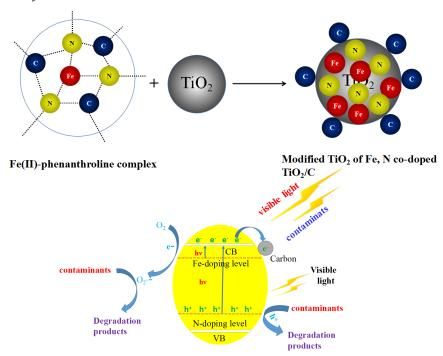
Inner and outer parts of TiO<sub>2</sub> were simultaneously modified to significantly improve its visible-light photocatalytic performance. This complicated modification was facilely fulfilled by a novel co-precursor method.
