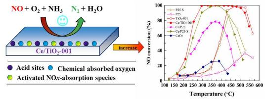
One-step synthesis of  $SO_4^{2-}$ -TiO<sub>2</sub> with exposed (001) facet promoted the formation of abundant acid sites, high concentration of chemically absorbed oxygen, and activated  $NO_x$ -absorption species, which were responsible for the SCR reaction.
