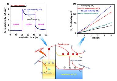
A gold nanoparticle/monolayer graphitic carbon nitride plasmonic photocatalyst prepared by a facile oil-bath method displayed a high photocatalytic hydrogen evolution rate of  $565 \, \mu \text{mol} \, \text{g}^{-1} \, \text{h}^{-1}$  because of the regulated flow of charge carriers.
