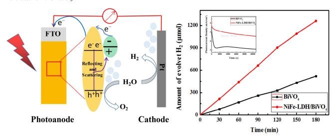
A high-performance BiVO<sub>4</sub> photoanode with a NiFe layered double-hydroxide nanoparticle cocatalyst was fabricated for photoelectrochemical water splitting. The cocatalyst boosted the photocatalytic activity, hydrogen production, and photoanode stability.
