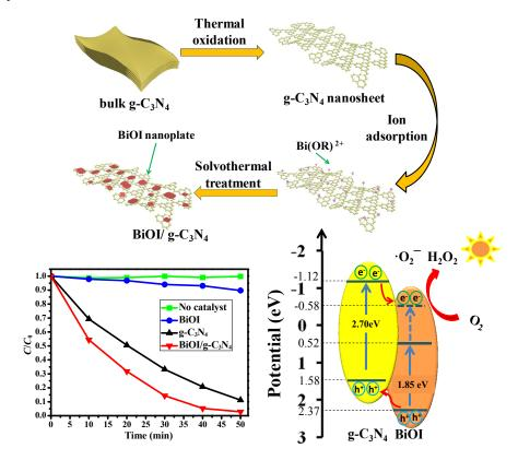
A BiOI/g- $C_3N_4$  nanosheet composite was constructed via in situ growth of BiOI nanoplates on the surface of g- $C_3N_4$  nanosheets. The composite showed excellent photocatalytic activity and recyclability under visible-light irradiation. A double-transfer mechanism of photoinduced electrons was proposed to explain the process of charge transfer and separation in the composite.
