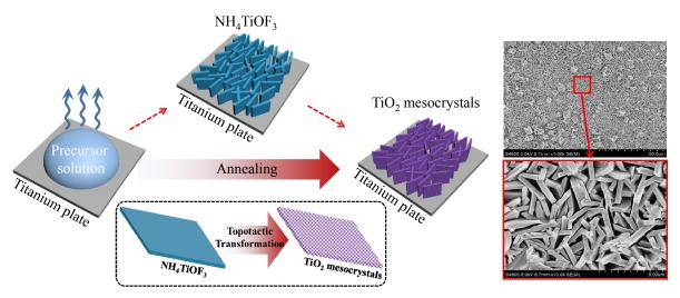
A TiO<sub>2</sub> mesocrystal film was successfully prepared by a direct annealing method. This new high efficient photocatalytic film electrode could be widely applied in photocatalysis and photoelectric catalysis.
