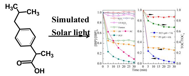
A synergistic PCF process was investigated for the degradation of ibuprofen at circumneutral pH. The IBP decay in the PCF process is much faster than that for the UV,  $UV/H_2O_2$ , Fenton, photo-Fenton and photocatalysis processes.
