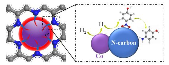
Cobalt nanoparticles encapsulated in N-doped carbon act as an efficient catalyst for room-temperature hydrogenation of nitroarenes owing to the synergetic effect of  $H_2$  activation on the Co nanoparticles and nitro group adsorption on N-doped carbon.
