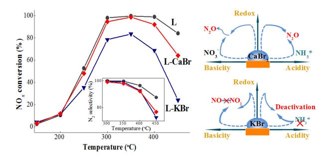
The decrease in the ratio of chemisorbed oxygen ( $O_{\alpha}$ ), reducibility and surface acidity contribute to the KBr-poisoned catalyst, and the overoxidation of NH<sub>3</sub> is attributed to the deactivation effect of CaBr<sub>2</sub> on the SCR catalyst.
