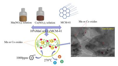
MCM-41 supported mixed oxides catalysts were synthesized by an impregnation method. The 10% MnCo (6:1)/MCM-41 catalyst showed the highest activity for chlorobenzene combustion.
