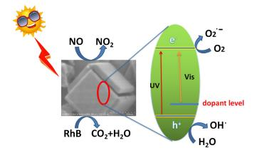
visible-light-driven N and S codoped TiO<sub>2</sub> hollow nanobox
