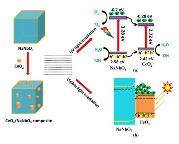
The  $CeO_2/NaNbO_3$  heterojunction composites were synthesized by a simple hydrothermal method. The formation of heterojunctions promoted the separation of photogenerated electrons and holes, thereby resulting in a higher the photocatalytic activity.
