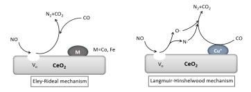
MO<sub>x</sub>-CeO<sub>2</sub> (M = Co, or Fe) catalysts mainly follow an Eley-Rideal reaction mechanism for the selective catalytic reduction (SCR) of NO by CO, whereas CuO-CeO<sub>2</sub> adopts a Langmuir-Hinshelwood SCR reaction mechanism in which the Cu<sup>+</sup> species ensure effective CO adsorption.
