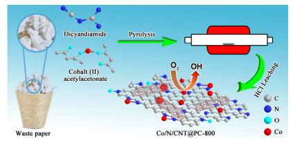
Paper-derived cobalt and nitrogen co-doped carbontube@porous carbon was fabricated as a nonprecious metal electrocatalyst and showed excellent catalytic performance for the oxygen reduction reaction.
