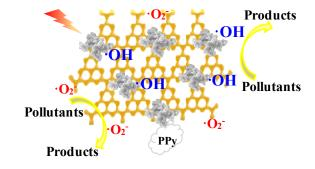
The degradation efficiency of methylene blue by PPy/g-C<sub>3</sub>N<sub>4</sub> composites synthesized by *in-situ* polymerization was three times higher than that of pure g-C<sub>3</sub>N<sub>4</sub>, where  $\cdot$ OH and  $\cdot$ O<sub>2</sub><sup>-</sup> radicals are the main reactive species.
