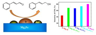
The doping of Fe to  $Ir/Mg_3Al$  could improve its activity and selectivity in cinnamaldehyde hydrogenation owing to the electronic interaction of Fe–Ir and the change in the geometrical structure of Ir active species.
