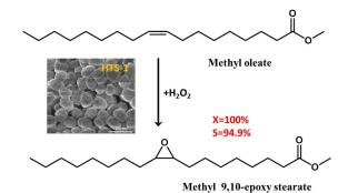
A high conversion of methyl oleate with  $\rm H_2O_2$  as a green oxidant was achieved using HTS-1 templated with polyquaternium-6.
