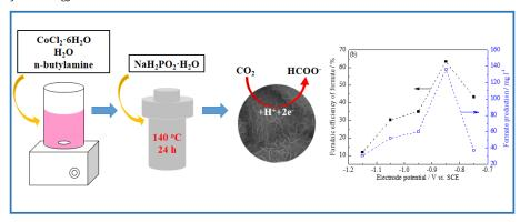
An efficient cobalt catalyst with unique flower-like morphology was synthesized by a facile hydrothermal method, which yielded a superior electrocatalytic activity towards CO<sub>2</sub> electroreduction with a high Faraday efficiency of formate (63.4%).
