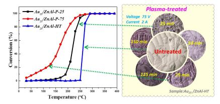
The protective ligands of supported gold nanoclusters could be effectively eliminated via atmospheric pressure non-thermal plasma treatment. This greatly enhanced their catalytic activity for CO oxidation.
