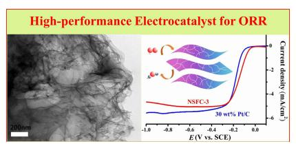
Nitrogen, sulfur and iron-tridoped mesoporous carbon nanosheets (NSFC) was fabricated using  $FeCl_3$  template from the protic salt PPS. The NSFC possessed comparable electrochemical catalysis with commercial 30 wt% Pt/C catalyst.
