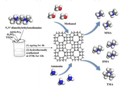
*N,N'*-dimethylethylenediamine was used as a template to synthesize DNL-6 with a high Si content, which showed excellent catalytic performance in the methanol amination reaction.
