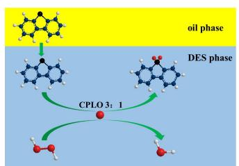
Sulfur compounds are extracted into the DES phase, where they interact. The carboxylic acid moieties of the DES are oxidized by  $H_2O_2$  to the corresponding peracids, which in turn oxidize the sulfur compounds to the corresponding sulfones.
