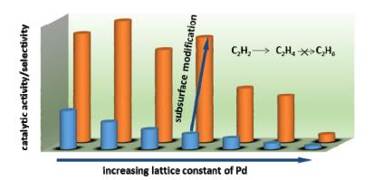
The effect of surface strain on the activity and selectivity of Pd and Pd-carbide for the hydrogenation of acetylene is thoroughly examined.
