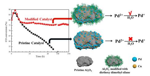
Support silylanization efficiently improved catalyst hydrophobicity and ensured stability after 150 h at 0  $^{\circ}$ C and 100% relative humidity. The detrimental role of water on stability through the inhibition of the production of the active Pd+ species was overwhelmingly restrained.
