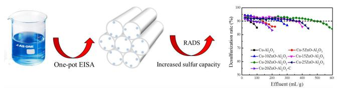
The ordered mesoporous Cu-ZnO- $Al_2O_3$  adsorbents were synthesized by one-pot evaporation-induced self-assembly strategy, which showed improvement in desulfurization activity and sulfur saturation capacity in reactive adsorption desulfurization (RADS).
