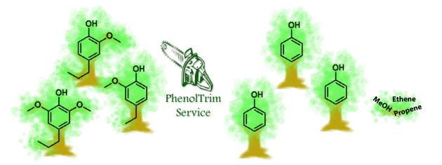
Lignin derived methoxyl alkyl substituted phenols were converted into phenol by hydro-demethoxylation and de-alkylation.
