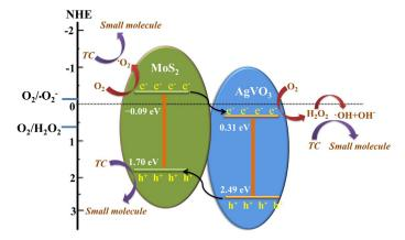
The  $AgVO_3/MoS_2$  composite photocatalyst was synthesized by the hydrothermal method. The excellent photocatalytic performance was due to the modification of  $MoS_2$  by  $AgVO_3$  which facilitated the  $O_2$  adsorption/activation and accelerated the two-electron oxygen reduction reaction for  $H_2O_2$  generation on the surface of  $MoS_2$ .
