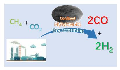
The developed encapsulated Ni/MCM-41 catalyst highly rendered metal sintering and carbon deposition at  $700\,^{\circ}$ C and exhibited long-term (200 h) high activity for DRM.
