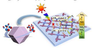
ZIF-8 was used as precursor for two-step calcination synthesis of ZnO nanoparticles with controlled OVs, which were used to effectively remove NO under visible light irradiation.
