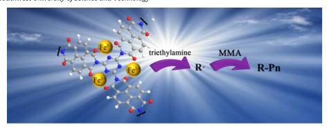
In this study, Fe(III) chelating melamine polyimide network (Fe@MPI) has been successfully synthesized and served as a heterogeneous catalyst for visible light driven radical polymerization of MMA. Fe@MPI can be easily separated from the polymerization solution due to its heterogeneous nature, and reused without losing its photocatalytic performance.
