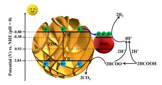
A novel  $MoS_2/Zn_3ln_2S_6$  ( $MoS_2/ZlS_6$ ) heterojunction photocatalyst was constructed with matching energy band potentials; it exhibited excellent performance in the excitation and transfer of photogenerated carriers and consequently, in visible-light-driven hydrogen production from formic acid.
