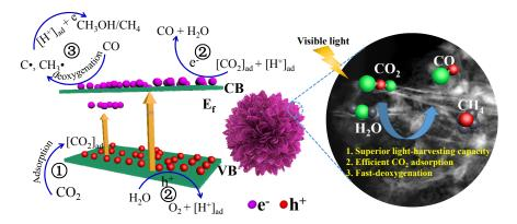
The as-prepared self-assembled  $Cd_{0.8}Zn_{0.2}S$  flowers with decorating ultrathin petals through an oil-bath method exhibit highly selective photocatalytic  $CO_2$  reduction under visible-light irradiation.
