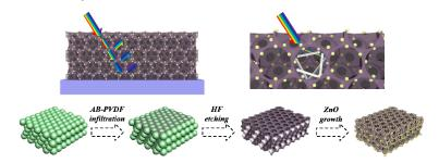
ZnO/PVDF inverse opal film was prepared to reach photothermal synergetic catalysis in the microreactor. By utilizing photon localization effect and slow light effect, the photocatalytic performance was greatly enhanced.
