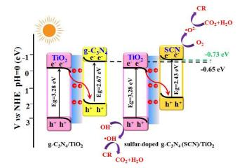
The S-doped g- $C_3N_4$  (SCN) possesses a stronger reductive performance than pure g- $C_3N_4$ . The S-scheme heterojunction formed by SCN and  $TiO_2$  can improve the separation efficiency of photoinduced electron-hole pairs as well as the photocatalytic activity.
