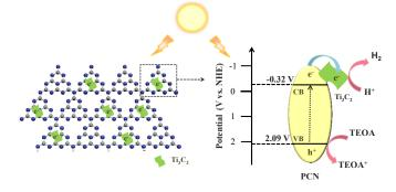
In addition to the protonation of graphitic carbon nitride, conductive 2D MXene was introduced as a co-catalyst to further accelerate electron-hole separation and interfacial charge transport for improved hydrogen production.
