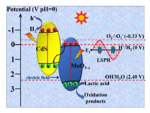
The  $MoO_{3-x}/CdS$  heterojunctions exhibit improved photocatalytic  $H_2$  generation activity, which is accredited to an LSPR-enhanced S-scheme charge transfer mechanism.
