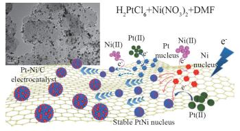
Highly monodispersed Pt-Ni/C alloy electrocatalysts were obtained through a facile electrodeposition method in *N*,*N*-dimethylformamide, which showed promising specific activity towards oxygen reduction reaction. The nucleation and growth mechanisms were explored through the comprehensive physiochemical characterizations as well as density functional theory calculations.
