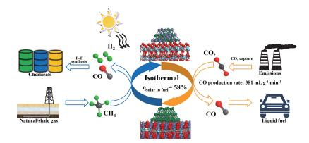
An unprecedented CO production rate of  $381~mL~g^{-1}~min^{-1}$  with  $99\%~CO_2$  conversion was achieved at  $850~^{\circ}C$  over an Fe-based oxide, with a theoretical solar-to-fuel efficiency of 58% in the absence of any heat integration.
