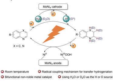
Water-involved transfer hydrogenation and dehydrogenation of N-heterocycles were developed by employing MoNi $_4$  as a bifunctional electrode. This method can be used to synthesize a series of functionalized hydrogenated and deuterated quinoxalines using  $H_2O$  and  $D_2O$ .
