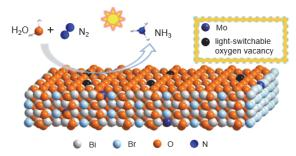
Enhanced ambient ammonia photosynthesis is achieved using Mo-doped  $Bi_5O_7Br$  nanosheets; these catalysts exhibit sufficient numbers of light-switchable oxygen vacancies serving as active sites, an optimized electronic structure, and a suitable absorption edge, resulting in enhanced  $N_2$  fixation photoactivity.
