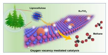
An "oxygen vacancy-mediated catalysis" was developed for the direct methanation of biomass with 82%-99% CH<sub>4</sub> yield from a wide range of biomass feedstock under  $200\,^{\circ}$ C.
