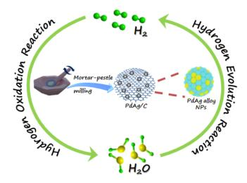
A facile grinding strategy is developed to produce a series of PdAg alloy NPs that are highly dispersed on various carbon supports. The resulting electrocatalysts exhibit excellent activities and stabilities in both the HOR and HER.
