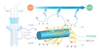
BUC-21/N- $K_2Ti_4O_9$  composites show high photocatalytic activity under UV and white light, which can be used to reduce Cr(VI) to Cr(III) effectively.
