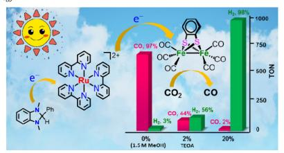
An [FeFe]-hydrogenase model was demonstrated to be highly active for the photochemical reduction of  $CO_2$  with a TOF of 7.12 min<sup>-1</sup> and CO selectivity of 97%. The  $CO/H_2$  ratio can be adjusted by the addition of TEOA.
