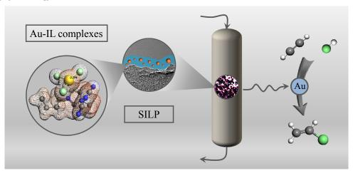
Cationic Au species coordinate with  $[Bmim][N(CN)_2]$  to form strong Au-IL complexes, which greatly increase the thermal and reaction stability of Au-based catalysts.
