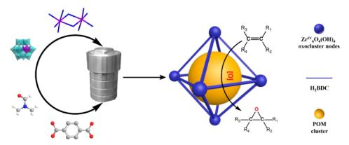
Hybrid composites based on Co-substituted phosphomolybdic acid ( $PMo_{11}Co$ ) and UiO-66 were synthesized by the direct solvothermal method.  $PMo_{11}Co@UiO$ -66 showed high catalytic activity and stability for the epoxidation of a variety of olefins with t-BuOOH as the oxidant.
