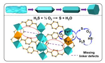
Using acetic acid coordination modulation, a series of MIL-53(Fe) with morphology evoluting from irregular bulky particles to highly uniform short hexagonal prisms were synthesized and applied for  $H_2S$  selective oxidation.
