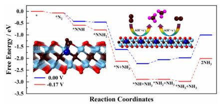
Single atom doped on MXene, which can synergize with the adjacent titanium atom on the matrix. With this synergy, the nitrogen reduction reaction can be proceeded at a low limiting potential.
