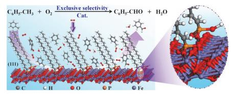
$HDPA-FeMO_x/\gamma-Al_2O_3$  is an enzyme-like catalyst for the exclusive conversion of toluene to benzaldehyde through  $O_2$  oxidation under mild conditions.
