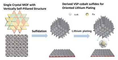
A single crystal metal-organic framework constructed by vertically self-pillared nanosheets has been prepared. Derived VSP-cobalt sulfides were employed for oriented lithium plating in metallic batteries.
