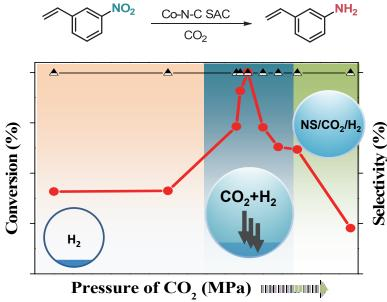
An inverted V-curve relation was observed between conversion and Pco2 in hydrogenation of 3-nitrostyrene over Co-N-C SACs in compressed CO<sub>2</sub>, where the peak was attributed to the enhanced solubility of H<sub>2</sub> in CO<sub>2</sub>-expanded substrate liquid.
