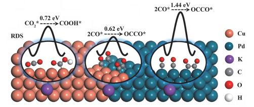
A CuPd(100) catalyst was designed and fabricated to improve the selectivity of the electroreduction of  $CO_2$  to C2 products by tuning the  $CO_2$  adsorption ability and intermediate reaction barriers.
