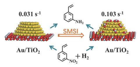
Strong metal-support interactions between Au and  $TiO_2$  can induce  $TiO_2$  invading the Au NP surface, accompanied by an enlarged perimeter. This effect can improve the hydrogen activation and boost the activity of the 3-nitrostyrene chemoselective hydrogenation reaction.
