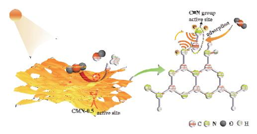
Cyano-modified porous g-C<sub>3</sub>N<sub>4</sub> nanosheets (MCN-0.5) with cyano groups as active sites exhibited enhanced photocatalytic activity for CO<sub>2</sub> reduction.
