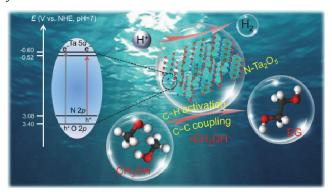
Photocatalytic activation of C–H bond within methanol to form hydroxymethyl radical ( $\bullet$ CH<sub>2</sub>OH) and subsequent C–C coupling to ethylene glycol (EG) with high selectivity and stability by co-catalyst free nitrogen doped tantalum oxide (N-Ta<sub>2</sub>O<sub>5</sub>) were reported.
