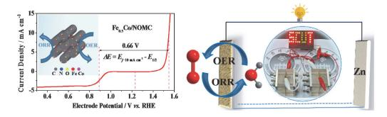
A robust ORR/OER oxygen-related catalyst was synthesized *via* a one-step method. A rechargeable zinc-air battery assembled using the optimal catalyst, *viz.* Fe<sub>0.5</sub>Co/NOMC, exhibits a power density of 153 mW cm<sup>-2</sup> at 1.0 V and superior cycling stability.
