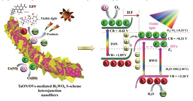
A novel  $TaON/Bi_2WO_6$  core-shell S-scheme heterojunction nanofibers with oxygen vacancies has been designed for highly efficient visible-light photocatalytic abatement of antibiotics and Cr(VI). The superior catalytic performance is benefiting from the efficient separation of high energetic charge carriers with optimal photo-redox power by S-scheme mechanism and rich oxygen vacancies, as well as the compact contact by the *in-situ* growth.
