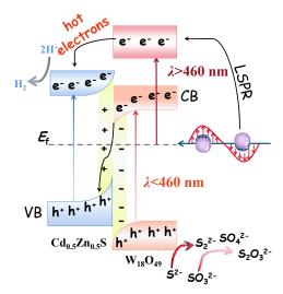
An ultraviolet-visible-near infrared induced extraordinary  $H_2$  evolution over  $W_{18}O_{49}/Cd_{0.5}Zn_{0.5}S$  photocatalyst based on the surface plasma effect and the S-scheme charge transfer.
