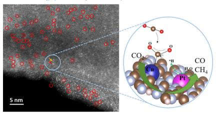
Atomically dispersed Pt-Cu sites inside crystalline carbon nitride were designed to maximize Pt mass activity and integrate their respective merits, leading to enhanced  $CO_2$  photoreduction.
