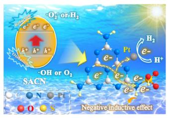
Sulfonic acid group-functionalized g- $G_3N_4$  has been synthesized successfully. The driving force generated by the negative inductive effect of sulfonic acid groups significantly improves the charge transfer dynamics and inhibits their recombination, thus leading to excellent photocatalytic performance.
