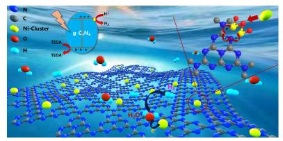
Monodisperse Ni-clusters were anchored on the CN surface for efficient photocatalytic hydrogen evolution. It has been proven that there is a stable interface interaction between monodisperse Ni-clusters and CN to construct the hybrid electronic structure of the Ni-cluster/CN system
