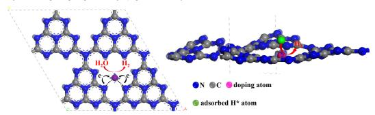
Atomic-level structural engineering of  $g-C_3N_4$  induced metal-N active sites in the framework and modulated the bandgap structure, thereby improving the separation efficiency of photogenerated charges, reductive ability, and light absorption.
