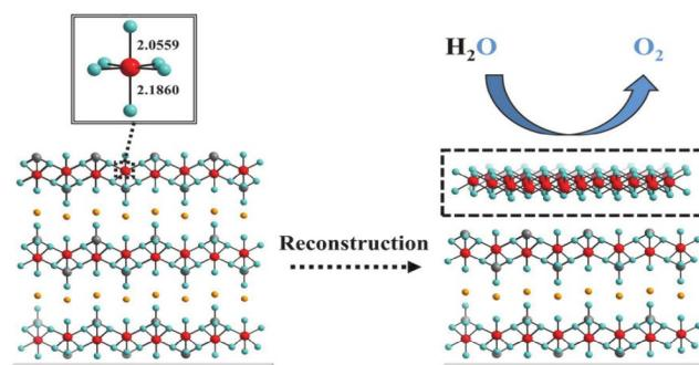
Two cobalt phosphates with distinct Co symmetry were obtained to explore the effect of coordination structure on the electrocatalytic oxygen evolution reaction. Asymmetric Co geometry can accelerate surface reconstruction to enhance OER activity.
