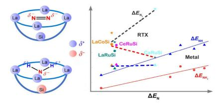
A bowl active site on the lanthanide intermetallic electride LaRuSi, composed of four surface La cations and one subsurface Si atom, plays the key role in efficient catalysis of  $N_2$ -to- $NH_3$  conversion by breaking the scaling relations through specific electrostatic and orbital interactions. This bowl active site thus presents a design concept of highly efficient heterogeneous catalyst for  $N_2$ -to- $NH_3$  conversion.
