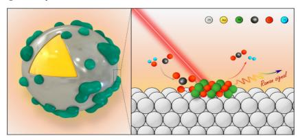
Direct spectroscopic evidence of the carbonate intermediate and its evolution during water-gas shift reaction at Pt-NiO interfaces is obtained using surface-enhanced Raman spectroscopy, based on which the reaction mechanism is then proposed.
