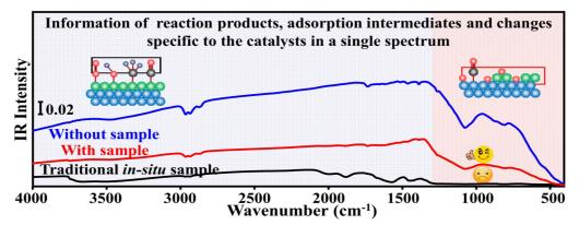
Surface adsorption intermediates and changes of the catalysts, as well as the formation products can be obtained in a single IR spectrum under reaction condition.
