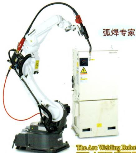
The Arc Welding Robot System
