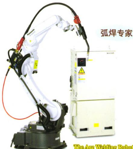
The Arc Welding Robot System
