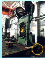
弹簧阻尼隔振器 Spring-damper vibration isolators
