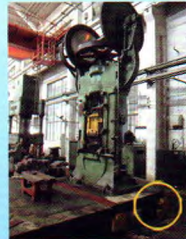
弹簧阻尼隔振器 Spring-damper vibration isolators
