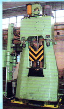
直接支撑的弹性隔振系统 Directly supporting spring vibration isolation system
