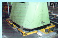
直接支撑的弹性隔振系统 Directly supporting spring vibration isolation system
