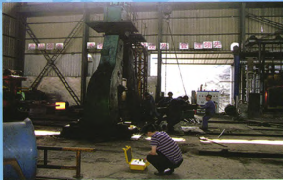
直接支撑的弹性隔振系统 Directly supporting spring vibration isolation system
