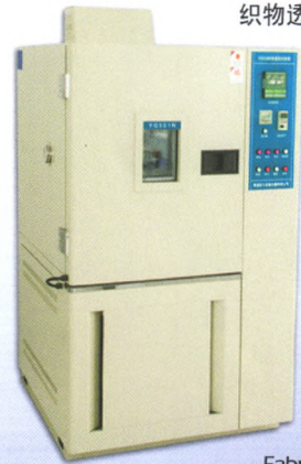
Fabric moisture permeability tester
