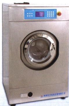
Fully automatic shrinkage tester
