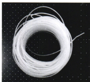
Filament used for FDM
