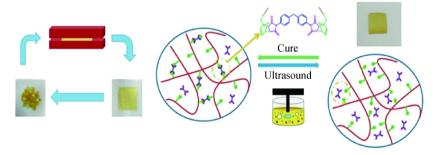
A series of polyetheramine (PEA) samples with self-healing and remolding properties were synthesized via Diels-Alder reaction. Hot press and ultrasound remolding approaches were conducted and studied in this system. After remolding for two generations, the regenerated PEA samples maintained above 70% of the original breaking strength and above 80% of the elongation at break. To be concluded, this series of PEA samples exhibited great performance on self-healing and remolding properties.
