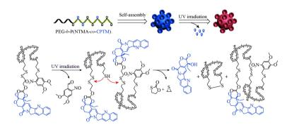
In the hydrophobic domains of the compound vesicles self-assembled from dual responsive PEG-b-P (NTMA-co-CPTM) amphiphilic polyprodrug diblock copolymer, mercapto groups could be decaged due to the photo-cleavage of the o-nitrobenzyl thioether moieties under UV irradiation, thus in-situ constructing reductive microenvironments. Then, CPT drug molecules were released via the exchange reaction between the decaged mercapto groups and the adjacent disulfide linkages.
