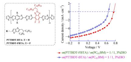
Two wide bandgap copolymers, PTTBDT-BTA and PTTBDT-FBTA, were prepared. Compared with PTTBDT-BTA, the 49.3% PCE enhancement of fluorinated PTTBDT-FBTA based device was benefited from simultaneous increases of Uoc, Jsc and FF.
