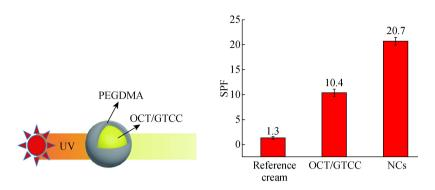
The biocompatible suncream nanocapsules loaded with OCT /GTCC were prepared by interfacial free-radical polymerization. Compared to the cream with the non-encapsulated OCT /GTCC, the cream containing NCs showed obviously higher SPF .
