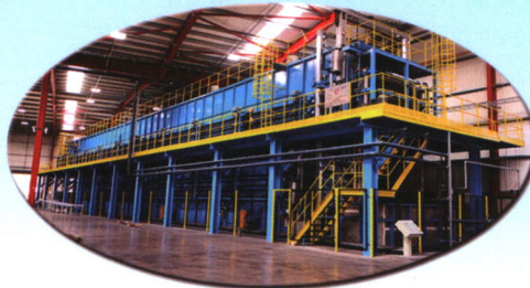
铝合金轮毂热处理生产线 Aluminum Alloy Heat Treatment Line for Wheels
