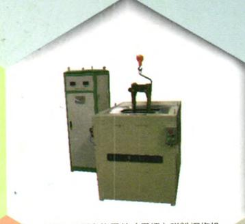
XGT-A型车钩零件(尾框)磁粉探伤机
