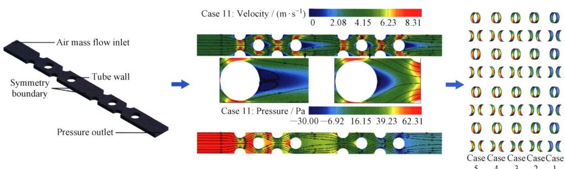
A three-dimensional model of eight rows wet air cooling plain tube bundle is established. And the mass source is applied to the tube surface to form liquid film based on the boundary condition of constant temperature. The Eulerian wall film model is coupled with the mixture species transport model to study the heat and mass transfer characteristics.
