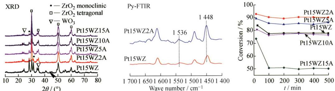
Al<sub>2</sub>O<sub>3</sub>-shaped catalyst PtWZA was prepared. Al<sub>2</sub>O<sub>3</sub> binder influenced the crystalline structure and acidity of the catalyst. The isomerization performance also varied with Al<sub>2</sub>O<sub>3</sub> binder loading. Moreover, the effects of Al<sub>2</sub>O<sub>3</sub> binder were very dependent on WO<sub>3</sub> content. The desirable shaped catalyst with high activity and high selectivity could be obtained.
