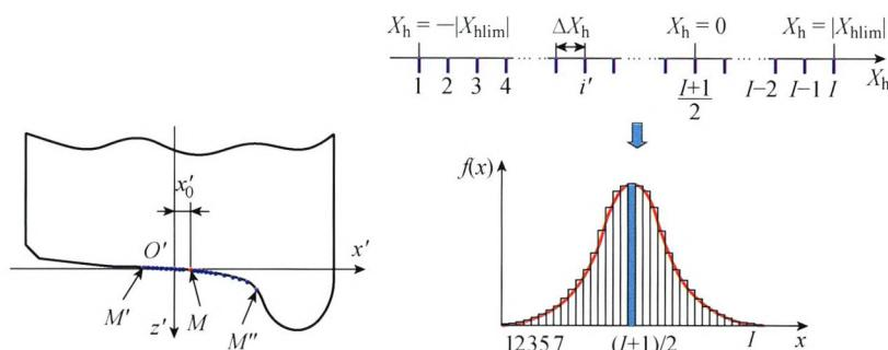
A method to calculate the fatigue life damage of wheel surface and predict fatigue life on actual railway is reported. The contact probability of wheel surface contact points after discretization is calculated by normal distribution. The methods of wheel rail contact stress calculation, fatigue damage accumulation hypothesis and fatigue curve equation are used in this study.
