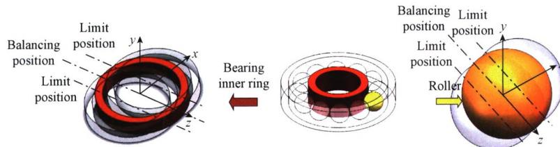
Taking deep groove ball bearing as the research object, the mechanical analysis is carried out. The noise calculation model for bearing is established, taking the bearing inner ring as the cylindrical sound source and the roller as the ball sound source. The influences of radial force and rotational speed on noise value are studied and discussed.
