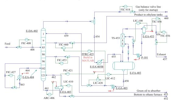
Dynamic simulation and optimization of ethylene distillation column (EDC) in its startup process is reported. EDC model built in Aspen HYSYS is integrated with startup operation strategy programmed in MATLAB to implement startup. An evolutionary algorithm is used to optimize startup strategy with the result of reducing energy by 25%.
