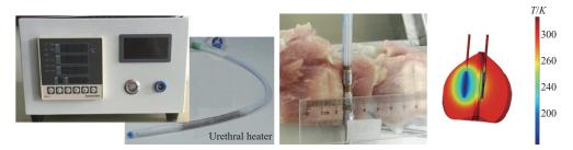
An effective temperature-controlled electrical urethral system was constructed. The precise 3D prostate models were established and combined with following experiments *in vitro* to verify its feasibility and controllability. This design facilitates the intelligent, rational and accurate control over temperature around the urethra in prostate cryoablation, reducing the negative impacts led by extra energy on the ablation area.
