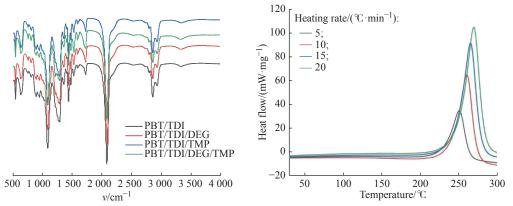
The results of Fourier Transform Infrared Spectroscopy (FT-IR) showed that the products of different curing systems had energetic azide polyurethane elastomer structure, and then the reaction kinetics and mechanical properties of different curing systems were studied.
