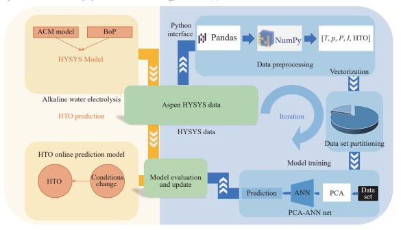
Overall framework of gas purity prediction model for alkaline water electrolysis system is based on PCA-ANN. HYSYS and Python interface are used for integrated training to realize online prediction and model iteration.
