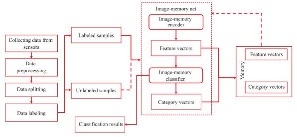
The labeled samples are used to train image-memory net which transforms time-series to feature vectors by image, and feature vectors are classified to category vectors by image-memory classifier. Then a memory mode is established with feature vectors and category vectors to classify the unlable samples.
