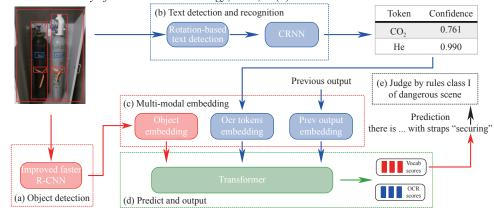
An image caption method combining multi-scale object detection and text detection recognition is proposed. It is shown from experimental results that the description statements generated by this method can effectively identify the dangerous substances and causes in the laboratory cylinder scene.
