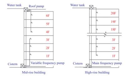
The energy consumption of secondary water supply operation under the two water supply modes is compared and analyzed, so as to provide technical reference for the later energy consumption reduction of water supply enterprises.
