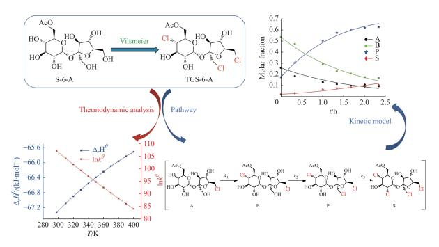
On the basis of thermodynamic analysis and reaction mechanism, a kinetic model of the chlorination reaction of S-6-A was established, and the kinetic parameters were obtained to guide the industrial process.
