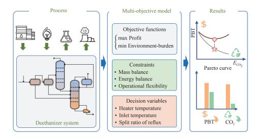
An integrated framework combining simulation and multi-objective optimization is proposed. An intelligent optimization algorithm is employed to solve the multi-objective optimization problem of the high and low pressure deethanizer process, and the TOPSIS method is used to obtain the optimal operating point on the Pareto front.
