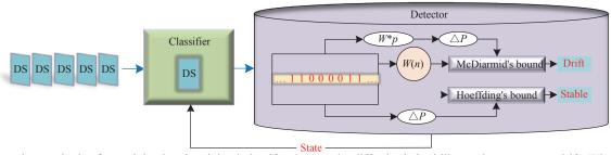
The detection methods of unweighted and weighted classification results differ in their ability to detect concept drift. When concept drift occurs, the unweighted method cannot detect the change in time, while the weighted method can quickly perceive the change and feed it back to the classifier.
