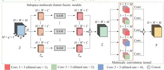
In the proposed subspace feature fusion module (SMFF), the sub-attention features of the sub-feature map in the spatial branch and the channel branches are calculated via the subspace attention module (SAM), and multi-scale convolution is performed on the output of SAM to enhance the correlation between sub-attention features.
