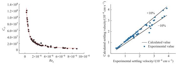
The relationship between drag coefficient and particle Reynolds number was analyzed to obtain a settling velocity model. The results showed that the error between experiment and model method was within 10%.
