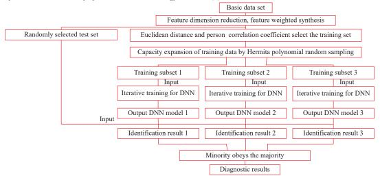
Firstly, the distributed depth neural network selects the fault characteristics through the mean and variance, then selects the training samples with the person coefficient and Euclidean distance, and finally predicts the fault through the principle of the minority obeying the majority.
