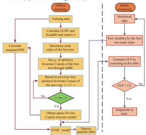
The proposed SDVC process monitoring scheme can overcome the nonlinear and non-Gaussian problem of high-dimensional data in industrial process, and achieve better fault monitoring performance and real-time performance than conventional D-vine Copula model.
