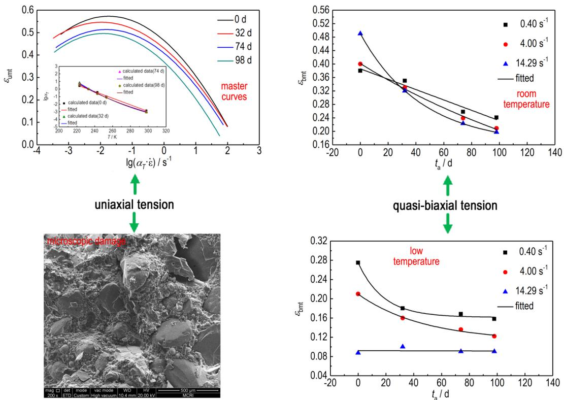
Failure criterion of three component HTPB composite solid propellants at low temperature under dynamic loading was proposed.
