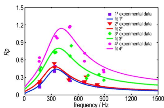
A new method for measurement of the nonlinear pressure coupling response function of solid propellants was established. The nonlinear pressure coupling response functions of three formulations of aluminum propellants were obtained. The characteristics of the nonlinear pressure coupling response of propellants were also analyzed in detail.
