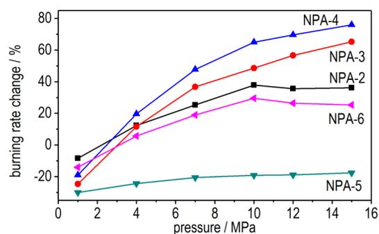
Several laboratory scale research on nitrate ester plasticized polyether (NEPE) solid propellants with and without ammonium dinitramide (ADN) and N-guanylurea-dinitramide (GUDN), featured with the same nominal composition, were prepared and evaluated. The combustion properties (strand burn rate and flame photos) and thermogravimetry (TG) analysis of propellants with ADN and GUDN were determined.
