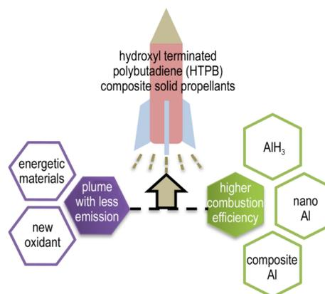
This review summarizes several typical new energetic materials (chlorine free oxidants) and novel Al-based composites materials that have been introduced to traditional hydroxyl terminated polybutadiene (HTPB) composite solid propellants.
