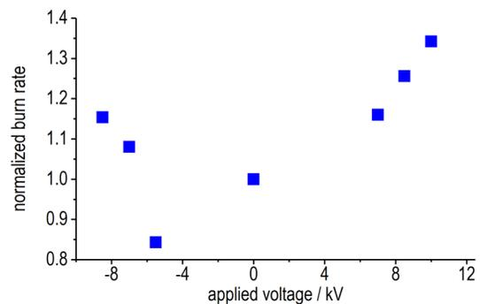
PMMA was used as the solid fuel for the study of electrical-ly controlled combustion under various electric fields.
