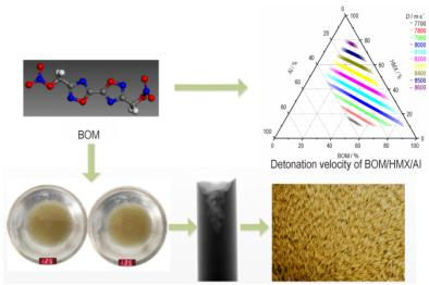
Thermal stability of BOM Defects of BOM casting sample Crystal morphology of BOM
