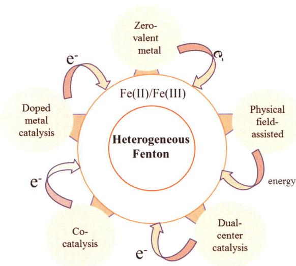
This paper summarizes the the mechanism of heterogeneous Fenton reaction, and the strategies of accelerating the cycle of Fe(III)/Fe(II).
