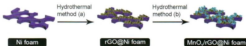
The  $\text{MnO}_2/\text{rGO@Ni}$  foam electrode is prepared by two-step hydrothermal methods with large surface area and outstanding electrocatalytic activity toward  $\text{H}_2\text{O}_2$  reduction.
