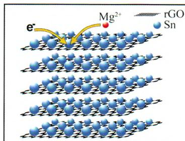
The 3D conducting network of rGO can effectively prevent the aggregation of Sn nanoparticles and alleviate the serious volume variation of Sn during repeated discharging/charging process. The Sn/rGO nanocomposite exhibits good capacity retention and a high Coulombic efficiency.
