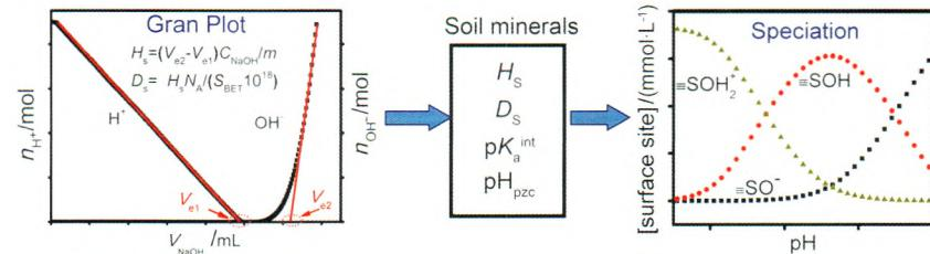
The acid-base property parameters of variable charge minerals were obtained by Gran plots with the 1-site/2-pK surface complexation model. These parameters, including their surface active sites concentration ( $H_s$ ) and density ( $D_s$ ), their acid-base equilibrium constants ( $pK_a^{int}$ ) and the charge zero  $pH_{pzc}$ , can reflect the acid-base buffer capacity of the soil minerals and further be used to predict the speciation distribution of red soil minerals under different pH.
