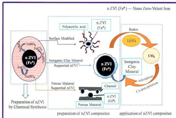
The summarization of recent research on the synthesis and application of nano Zero-Valent Iron nanocomposites for the efficient removal of radioactive uranium from environment.
