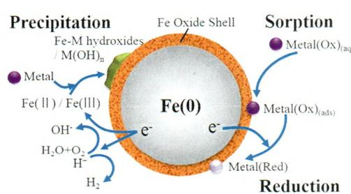
Nanoscale zero-valent iron (nZVI) is a perfect example of core-shell structured and multifunctional nanomaterials for environmental applications, and has rich surface chemistry. The unique core-shell structure and the surface chemistry endow nZVI with unique and multi-faceted functions for heavy metal removal including sorption, reduction and precipitation.
