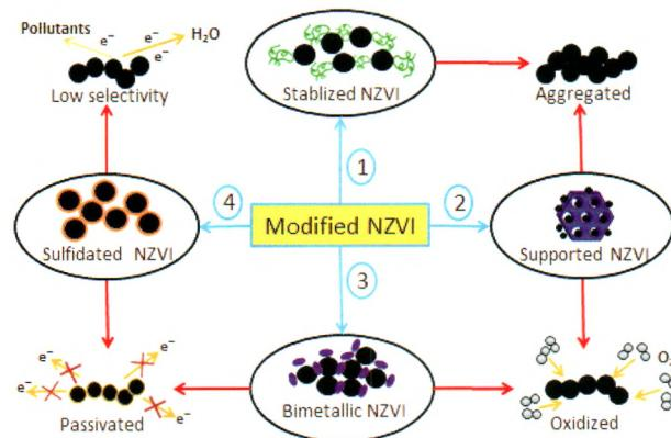
Among different modification strategies, sulfidated nanoscale zero-valent iron shows enhanced reaction activity and electrons selectivity in treating aqueous pollutants.
