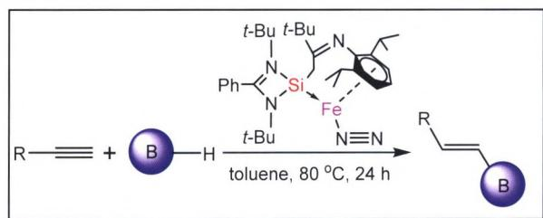
The neutral silylene-imine iron(0) dinitrogen complex enabled catalytic hydroboration of terminal alkynes.
