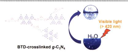
Conjugated crosslinking modification of graphitic carbon nitride with benzothiadiazole improves visible light-driven photocatalytic hydrogen production from water.
